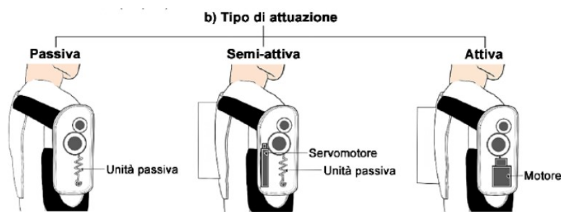
Figure 1.4. Exoskeleton Categorization by Actuation Type [11]
