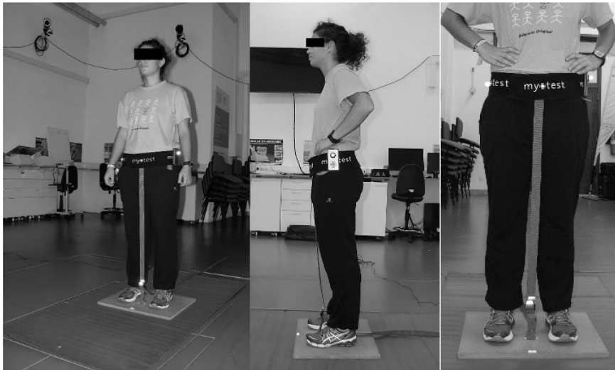
Figure 2.2: An example of a combined marker-based + force plate experimental setup. Image obtained from Conceição, Lewis et al. [27] «An Evaluation of the Accuracy and Precision of Jump Height Measurements Using Different Technologies and Analytical Methods» under creative commons license.
