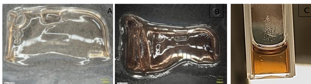
Figure 5.5 Cured objects obtained with Xube 2 (A) 0.02% IOPs, 50\text{-}52.5 \text{ mJ/mm}^2 (B) 0.02% IOPs, 55 \text{ mJ/mm}^2 (C) 0.03% IOPs, 60 \text{ mJ/mm}^2
