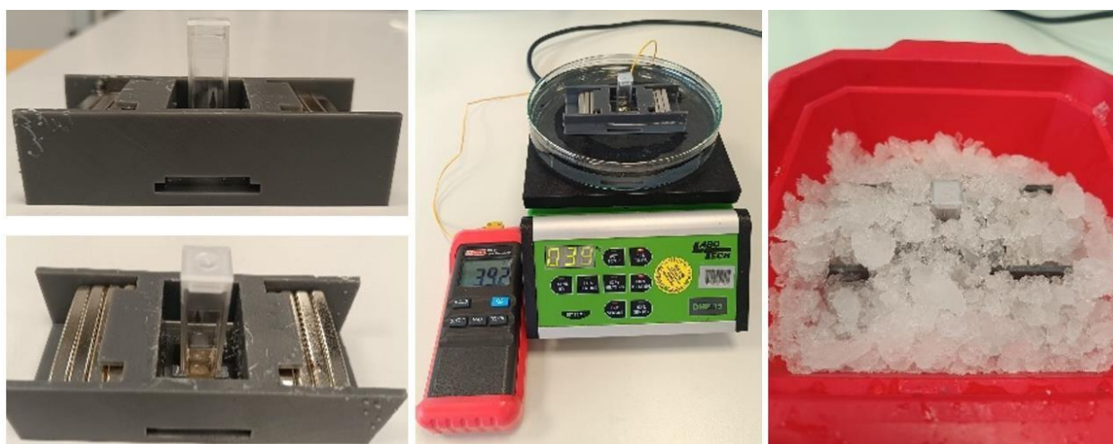
Figure 4.9 Left: picture of the assembled system: holder, magnets and cuvette; Center: Assembled setup placed in the warm water bath during the IOPs self-assembly; Right: Assembled setup immersed in ice to promote thermal gelation of the composite photoresin
