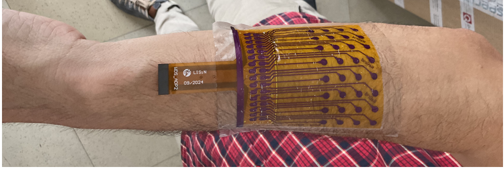
Figure 3.4: Placement of the thin-film, ultrasound-transparent electrode array on the forearm, featuring 32 electrodes in a 8x4 matrix. The array is positioned over the EDM muscle, with columns (8 electrodes each) oriented perpendicular to the muscle fibers and rows (4 electrodes each) aligned along the fiber direction.
