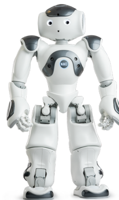
Figure 2: NAO - Humanoid robot (SoftBank Robotics, s.d.)
