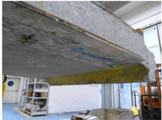
Figure 29: Left: Construction joint between span 2 and span 1. Right: Efflorescence in span 1
