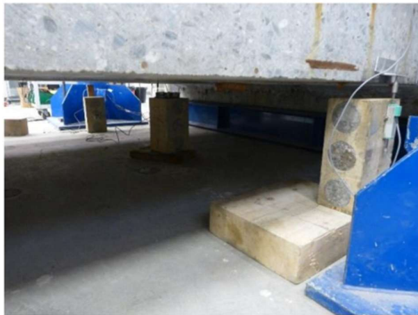
Figure 18: Sensors positioned to monitor settlement at load application points
