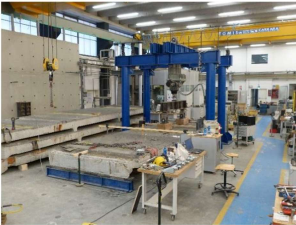
Figure 12: General view of the test setup for scheme 2 and load cell detail
