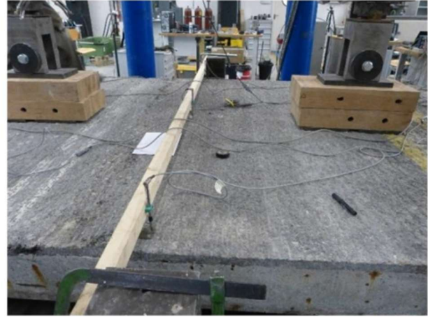
Figure 17: Sensors positioned to monitor the failure of the internal supports
