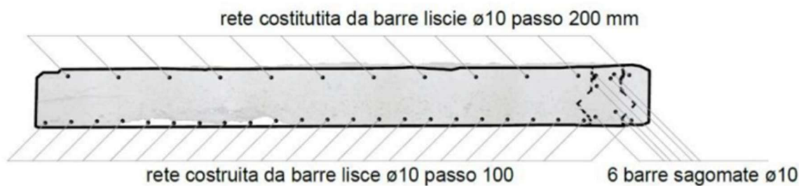
Figure 73: Reinforcement layout in lateral prefabricated segment
