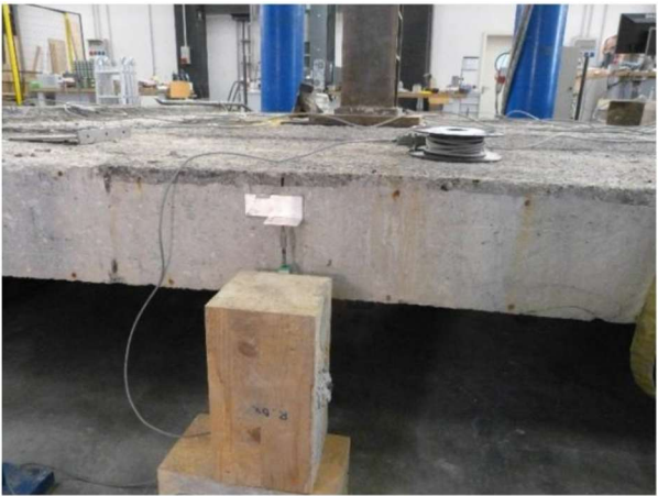
Figure 43: Significant crack pattern on the front of the slab
