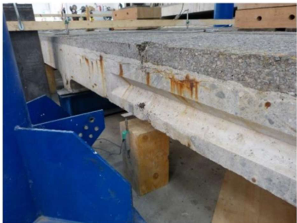
Figure 30: Left: Small demolitions near loading point of span 2. Right: Crack pattern at span 3
