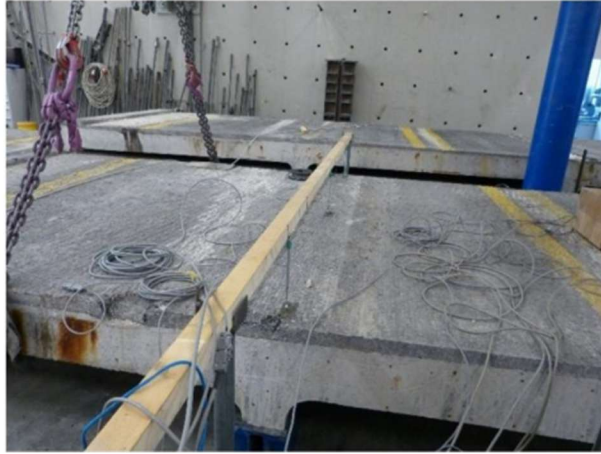
Figure 17: Sensors positioned to monitor the failure of the internal supports
