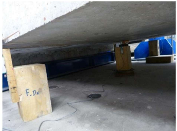
Figure 18: Sensors positioned to monitor settlement at load application points
