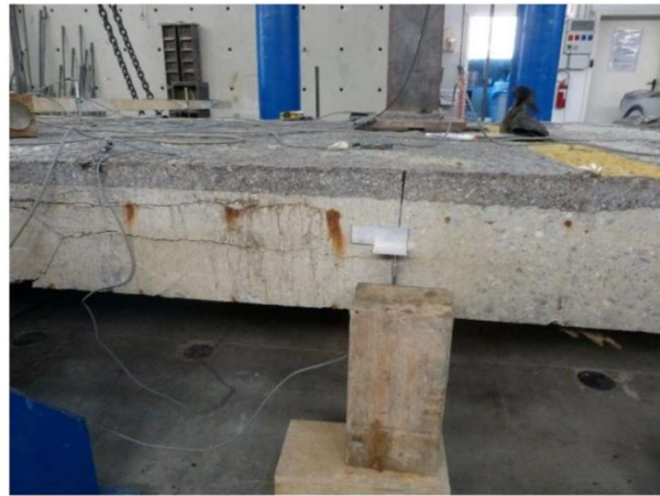
Figure 43: Significant crack pattern on the front of the slab
