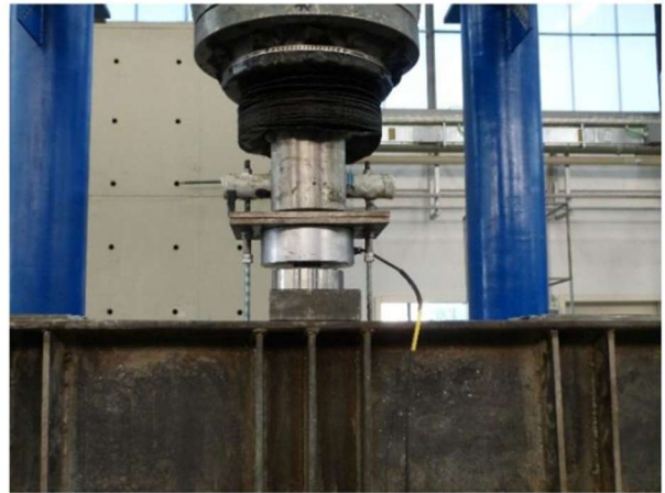
Figure 12: General view of the test setup for scheme 2 and load cell detail
