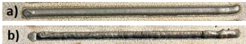
Figure 20: Manufactured single layer beads: a) good manufacturing, b) lack of fusion.
