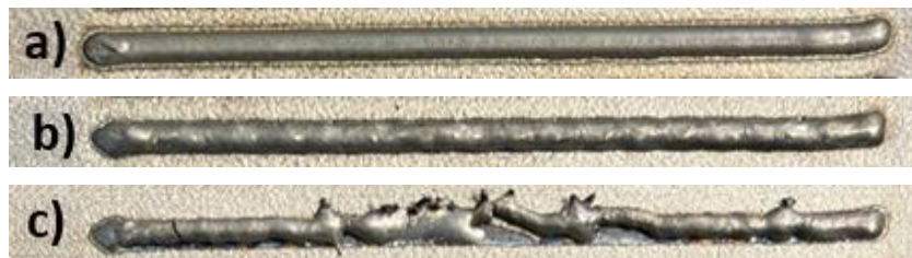
Figure 18 : Manufactured single layer beads: a) good manufacturing, b) moderate stubbing c) excessive stubbing.
