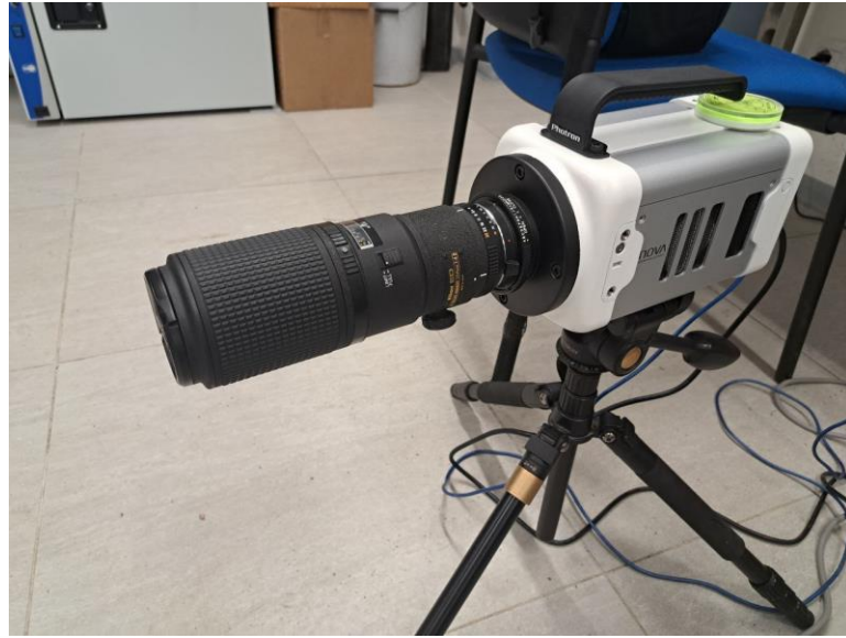
Figure 9 High-speed camera setup (Photron FASTCAM Nova S16) used for cavitation bubble observation.
