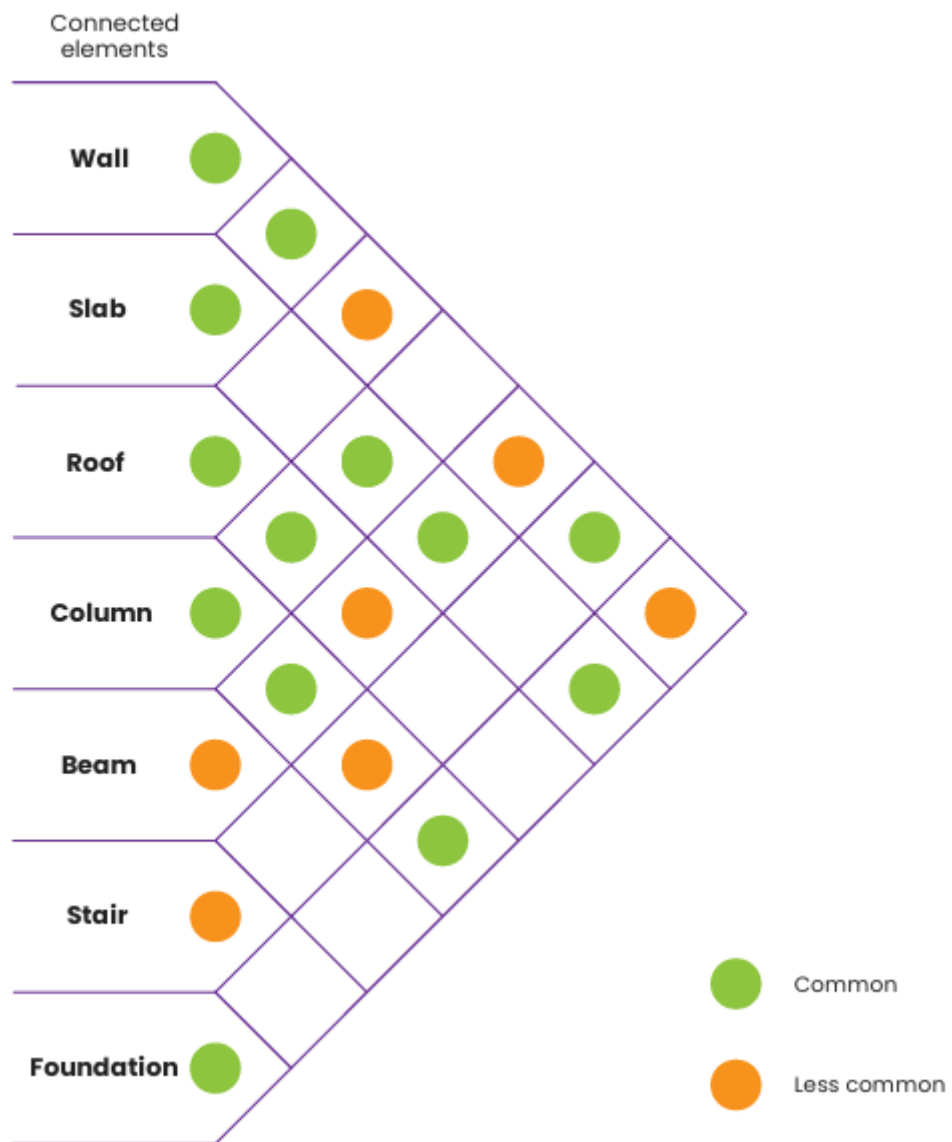
Figure 35 Diagram showing the most common component-to-component connections.
