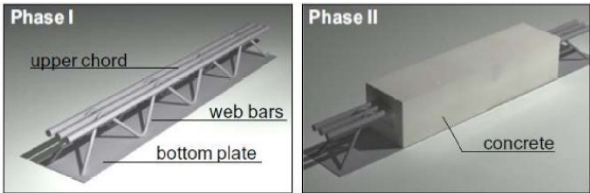
Figure 87 Beam structural schemes in operating Phases I and II.
