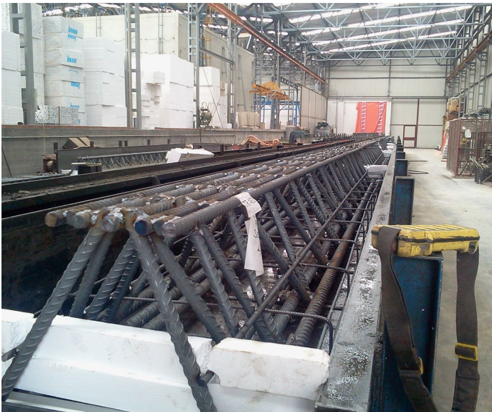
Figure 121 Picture from “U.T. FORNACE CALANDRA s.r.l.” production where is shown a CSTCB assembled in the factory.
