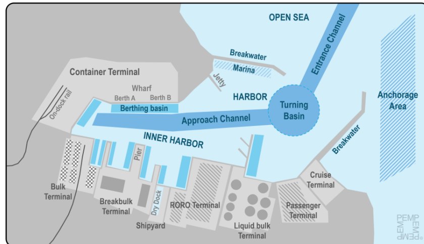
Figure 2: Fundamental physical elements of a port [14]
