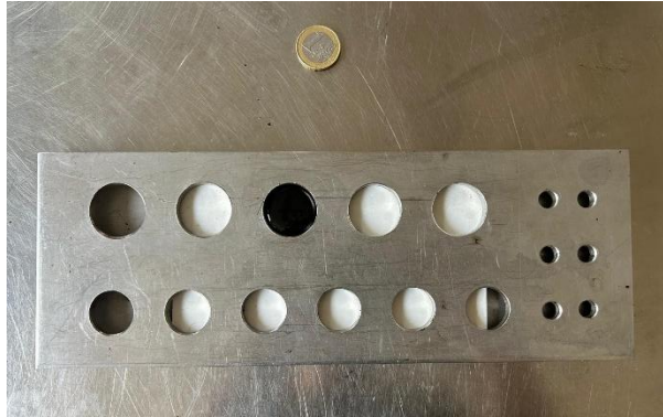
Figure 93 - System for preparing 3 mm gap specimens
