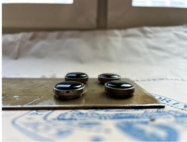
Figure 65 - Pouring of bitumen into the brass rings (slightly excessive amount)
