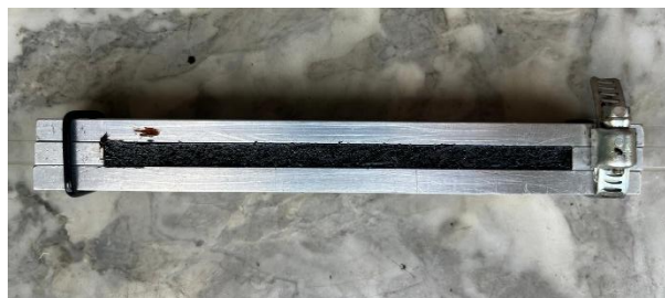
Figure 82 - Trimmed specimen for BBR test
