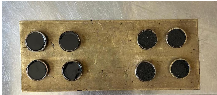
Figure 66 - Leveled bitumen specimens after excess removal with a heated spatula
