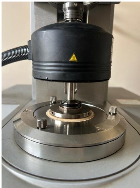
Figure 94 – Positioning of the sample with 3 mm gap
