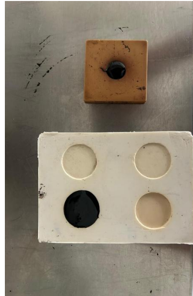
Figure 87 - Bitumen sample after heating process
