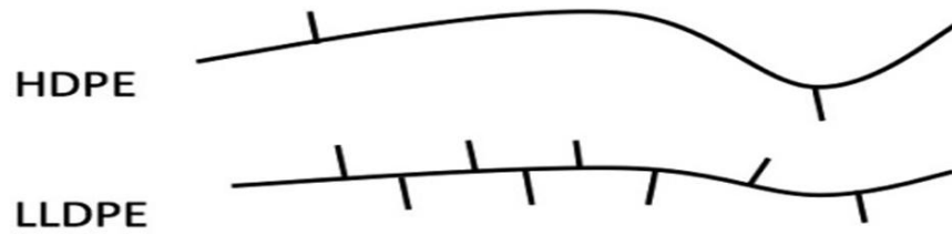
Figure 8 - Chemical structure of HDPE and LDPE [9]
