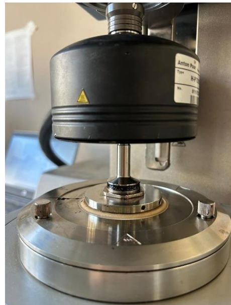
Figure 95 – Trimmed sample with 3 mm gap
