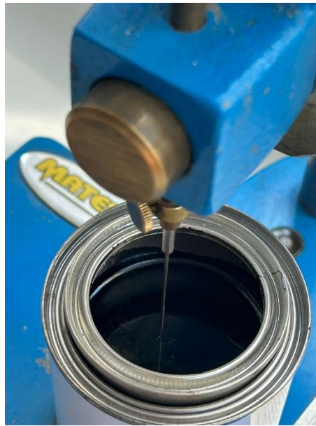
Figure 63 - Positioning of the needle for the penetration test
