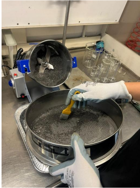
Figure 50 - Manual sieving of the fragmented sample using a 1 mm sieve
