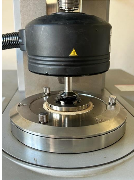
Figure 92 - Melted specimen during DSR test
