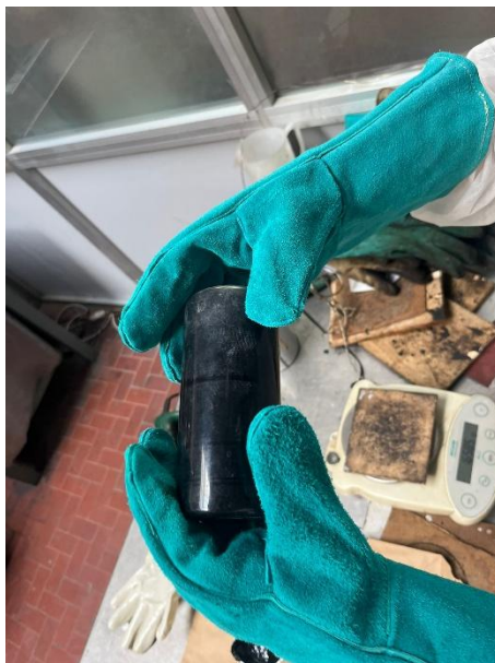
Figure 72 - Preparation of the film for RTFOT
