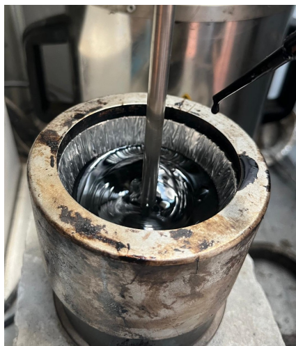
Figure 3.12: Addition of the rejuvenator using a pipette.
