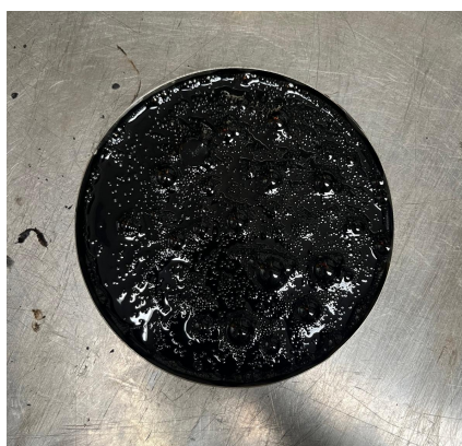
Figure 3.9: Pan filled with PAV aged bitumen.
