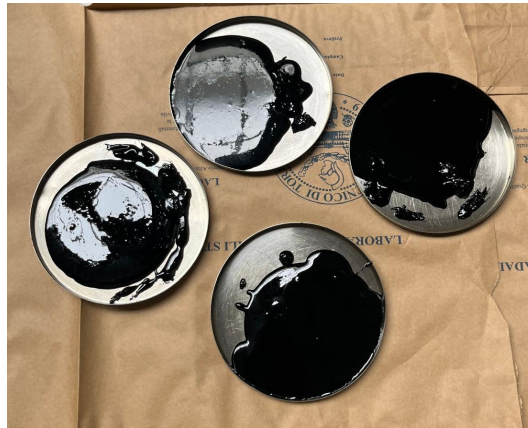
Figure 3.7: 4 PAV pans filled with 50 g of RTFOT aged bitumen.
