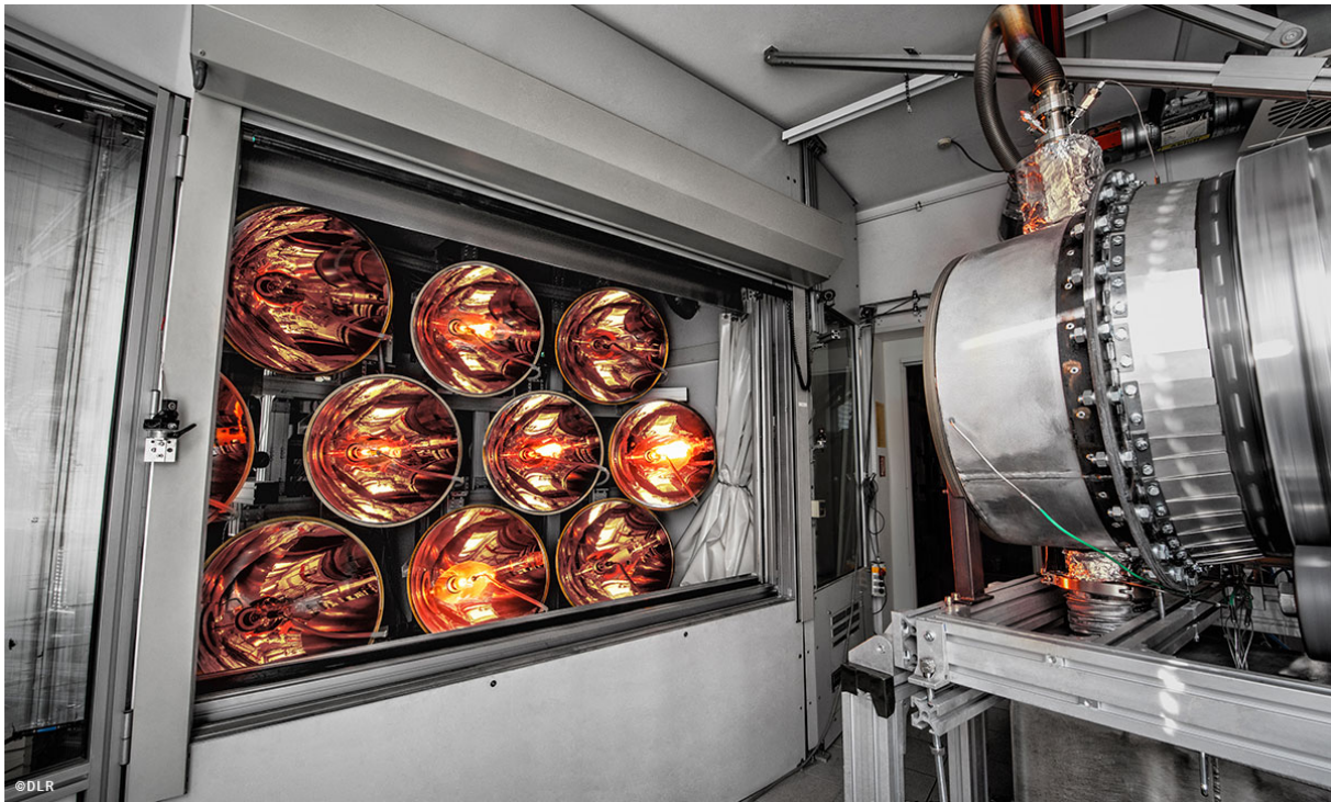
Figure 2.6: Xenon lamps used in the spotlight facility in Cologne for rotary kiln testing[24, 5].
