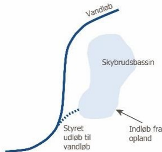
Figure A.2: Schematic representation of cloudburst pools [28]
