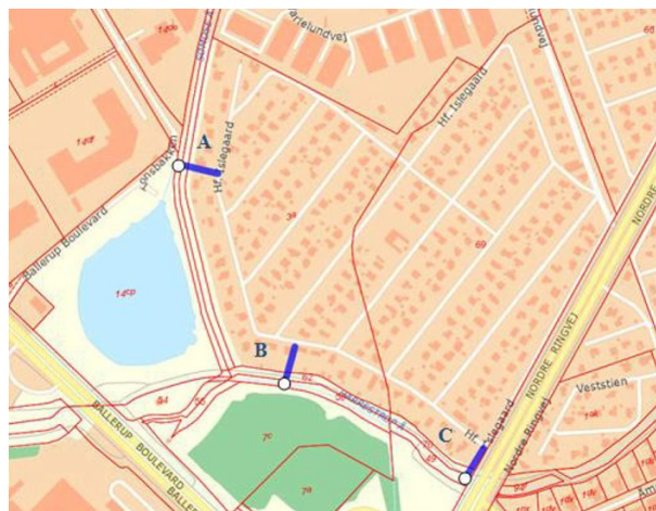
Figure 5.12: Three water diversions into the Sømose and Harrestrup Rivers [29]
