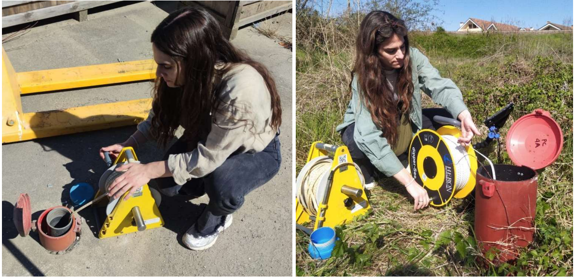
Figure 20. Depth to water level measurements using a water level meter (left) and well video-inspection (right).
