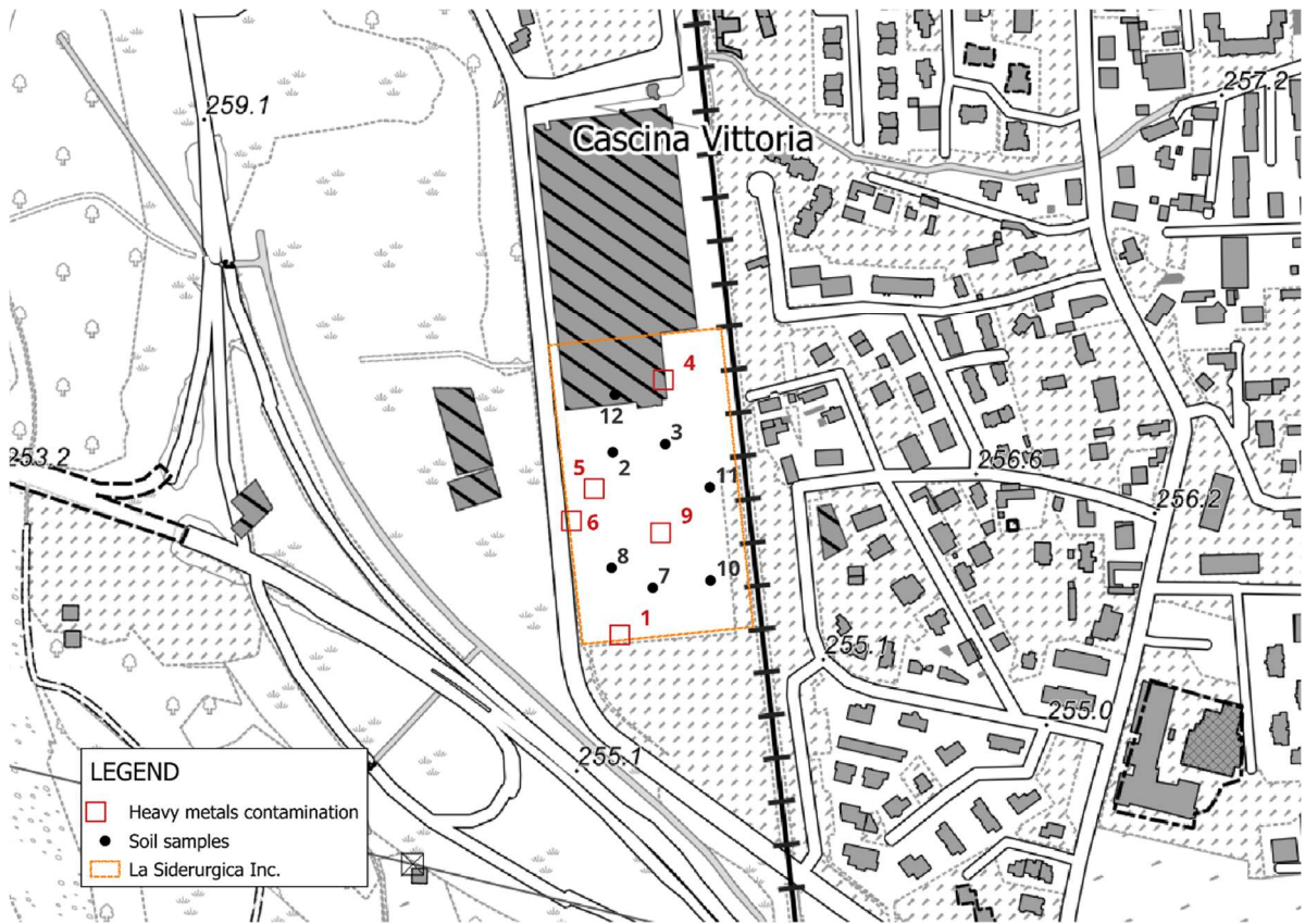
Figure 7. Location of soil sampling points related to the 1999 soil contamination.
