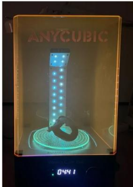
Figure 28- Face Mask mold- Version B TR300- placed inside the UV curing system during the post-curing process.
