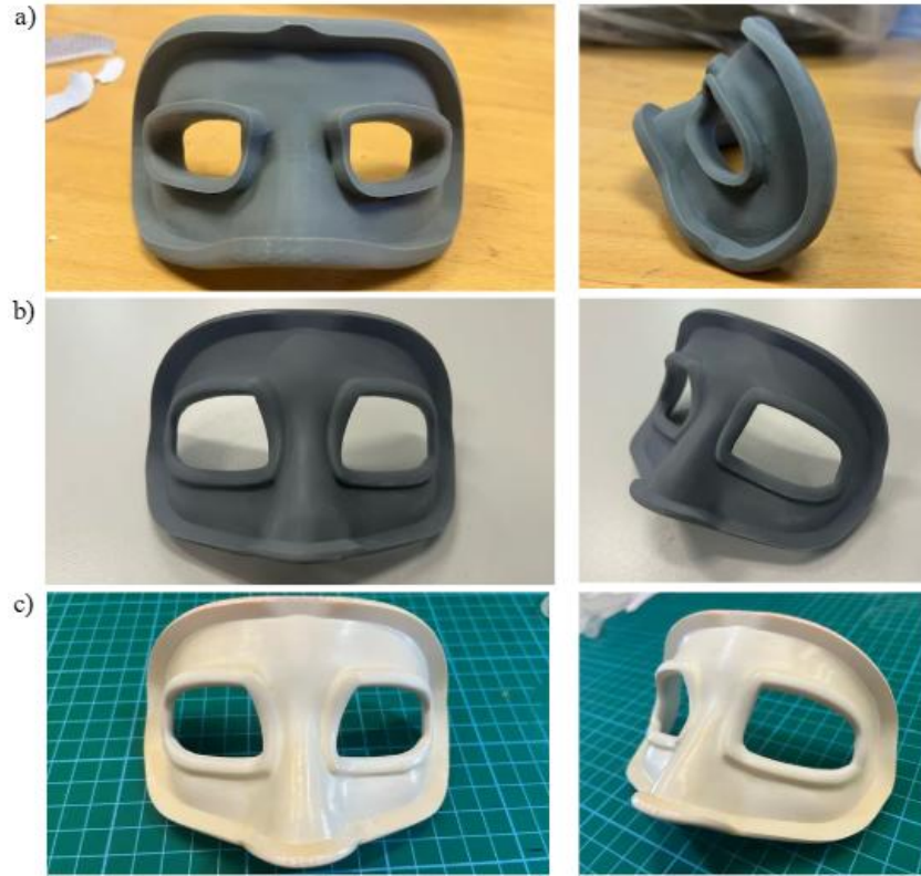
Figure 26- Fabricated Face Mask molds: (a) Version A printed in TR300 resin; (b) Version B printed in TR300 resin; (c) Version B printed in Ceramic Pro resin.
