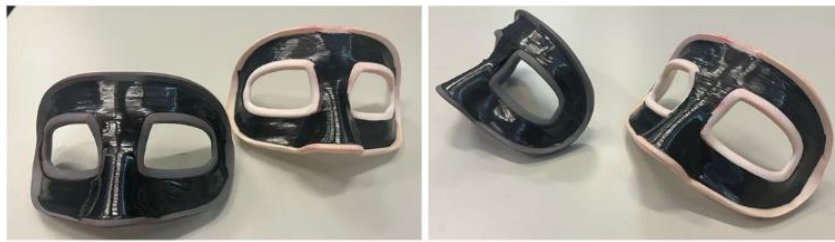
Figure 35- Face Mask Mold- Version B - after completion of the lamination, with all prepreg layers applied.
