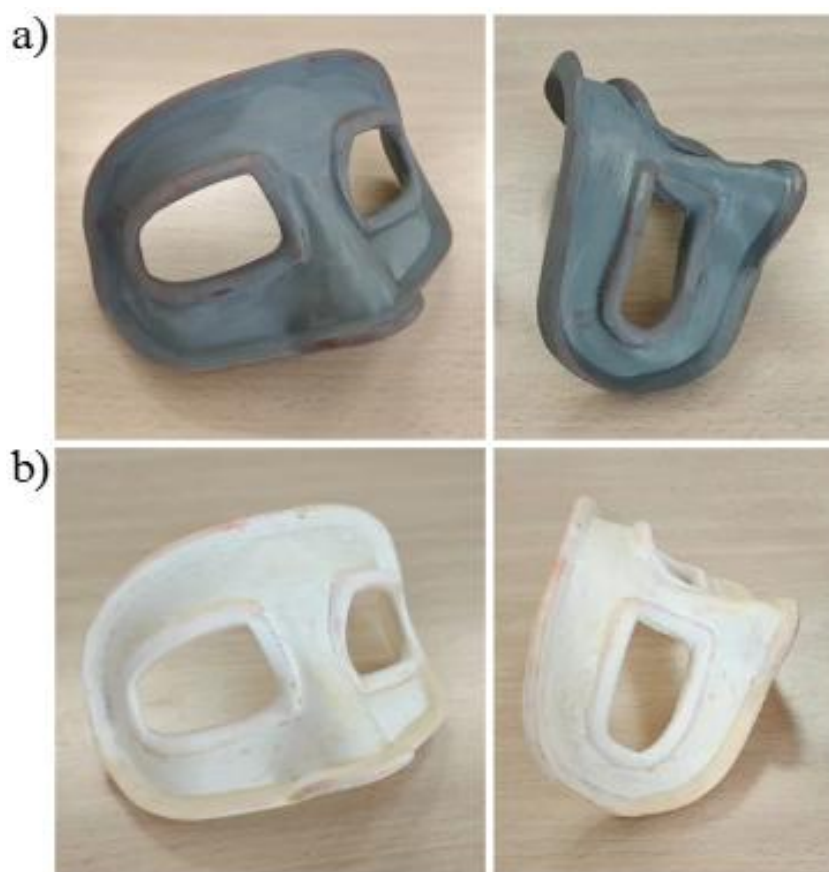
Figure 45-Face Mask mold- version B- after curing cycle in Autoclave. a) TR300, b) Pro Ceramic.
