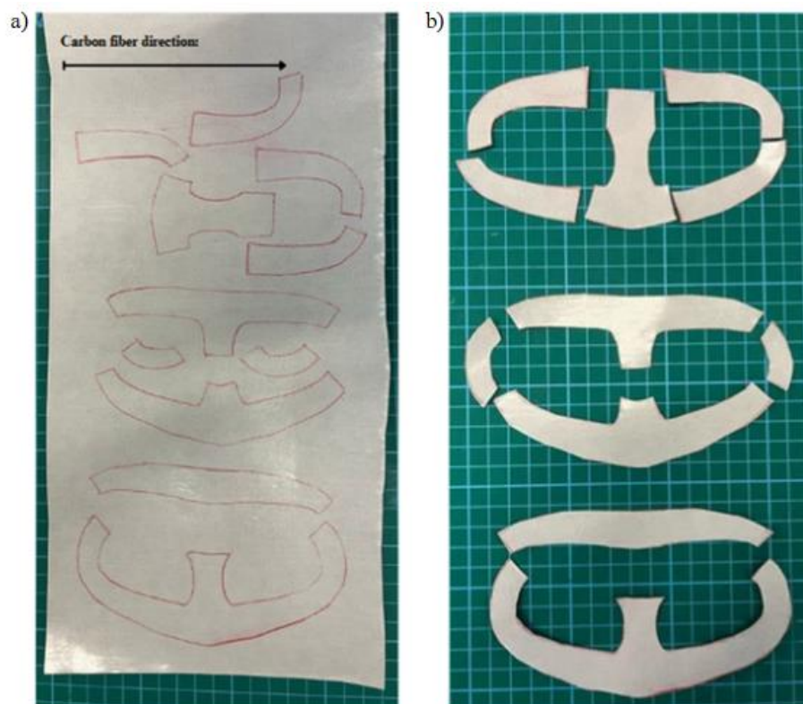
Figure 32- (a) Drawing of the ply patterns to be cut from the prepreg sheet; (b) corresponding cut pieces ready for lay-up.
