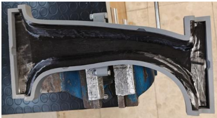
Figure 36- B.pillar Mold after completion of the lamination, with all prepreg layers applied.
