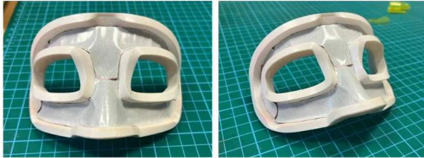
Figure 33- Dimensional verification of the cut prepreg pieces while still covered by protective polymer films.
