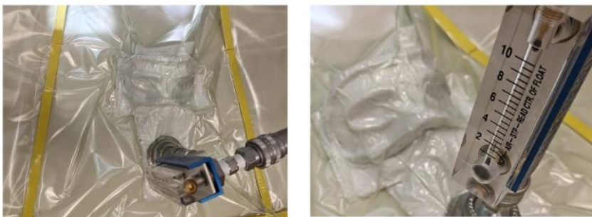
Figure 38- Vacuum system functionality check.
