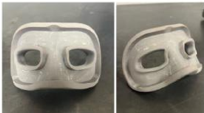
Figure 44- Face Mask mol- version A- after curing cycle in Autoclave
