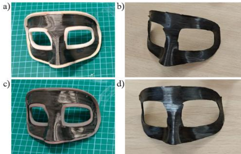
Figure 42- Facial orthosis mask – version B: (a) Component inside the mold – TR300 resin, (b) Component after demolding – TR300 resin, (c) Component inside the mold – Pro Ceramic resin, (d) Component after demolding – Pro Ceramic resin.
