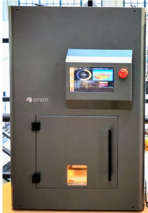
Figure 3-1: Orion A150 AM printer
