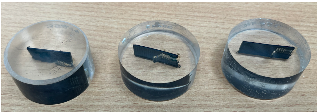
Figure 3-8: Samples for microscope analysis
