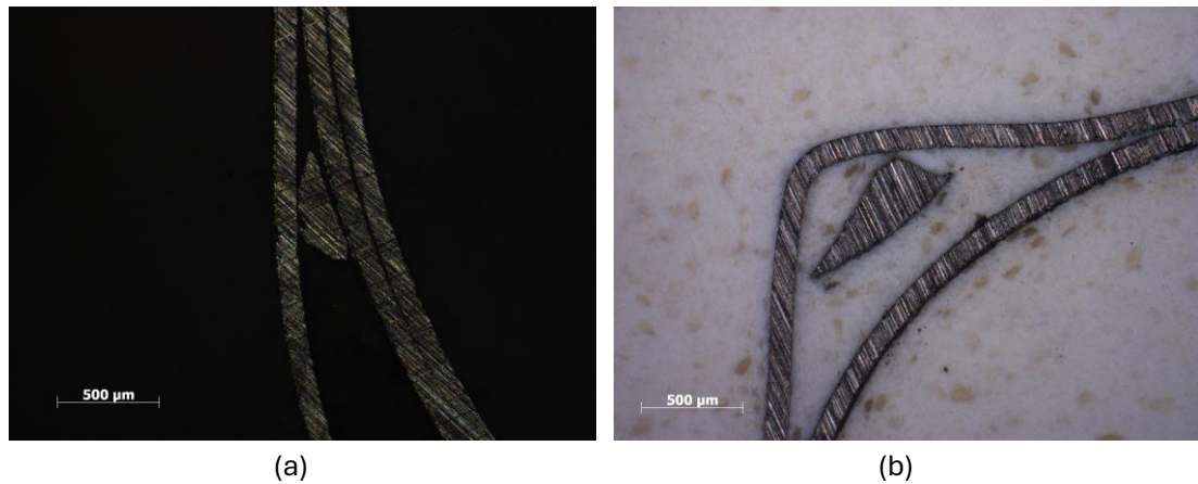
Figure 3.12 Chip sample collection of a) AISI 4140 b) 316L SS
