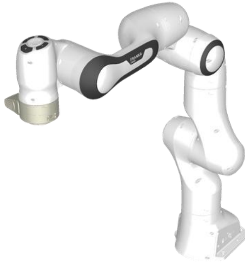
Figure 3.3. Diagram of Franka Emika Panda Cobot [41]
