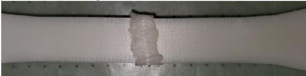
Figure 2.9. ABS broken specimen repaired with fused filament by 3D printing pen, following “U” deposition pattern [25]
