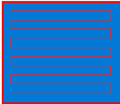
Figure 3.36: Melt theme beam trajectory
