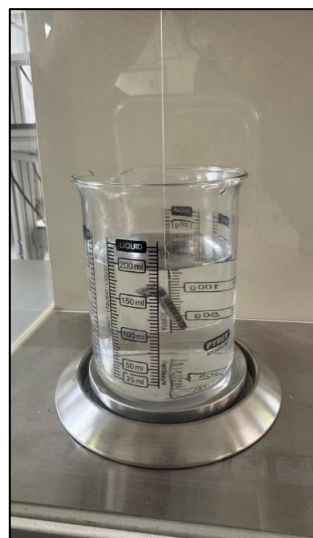
Figure 3.56: Physical set-up for measuring density
