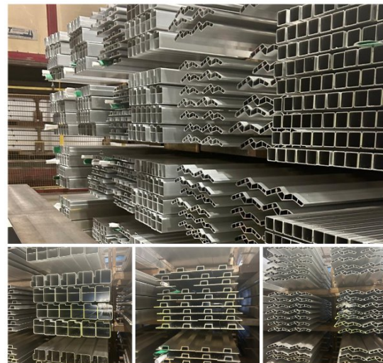
Figure 3.3 : Multi-chambered Aluminum profiles
