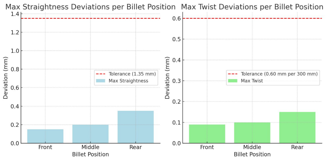
Figure 4.31 : Max Deviations per Billet Position Straightness and Twist
