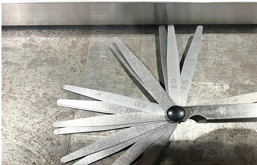
Figure 3.1 : Feeler gauges (0.01 to 1.00 mm)
