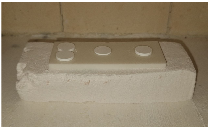
Figure 4.5: Sintered LAMGP pellets.
