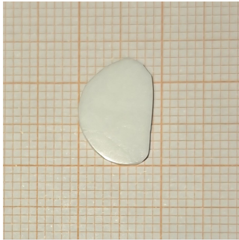
Figure 4.4: Reshaped and polished bulk LAMGP specimen.
