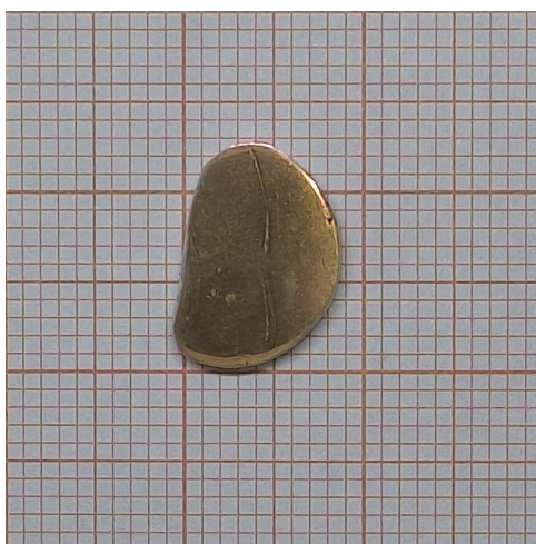
Figure 4.6: Sample prepared for electrochemical testing.
