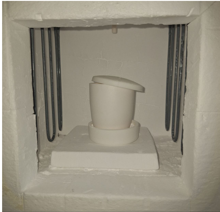
Figure 4.2: Furnace setup for glass casting.
