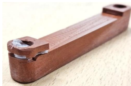
Figure 5.13. HTPLA insert after removal from the mold
