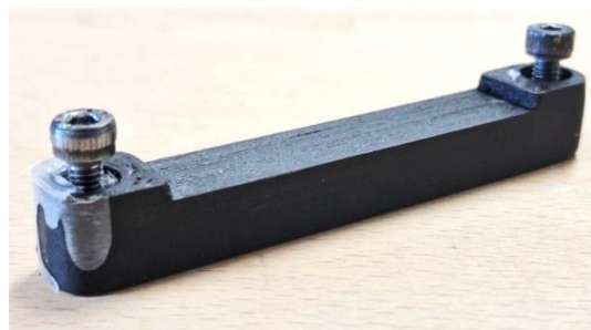
Figure 5.9. Carbon PA insert after removal from the mold
