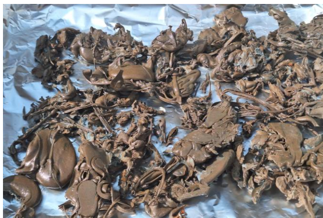
Figure 3.43. Material removed from the Brabender after compounding
