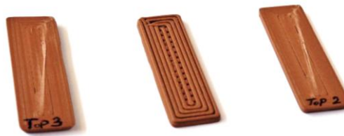
Figure 3.16. HTPLA samples printed for DMA test
