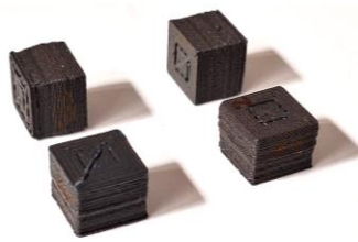
Figure 3.49. PLA–Copper 60% samples printed for compression test
