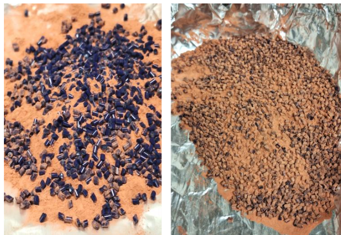
Figure 3.41. Preparation and manual mixing of PLA with copper powder
