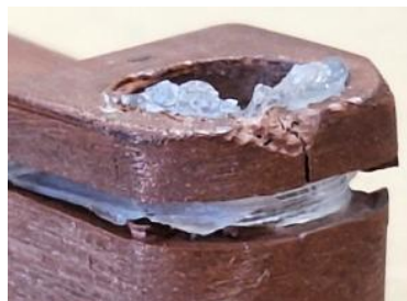
Figure 5.17. Copper Filament insert after removal from the mold
