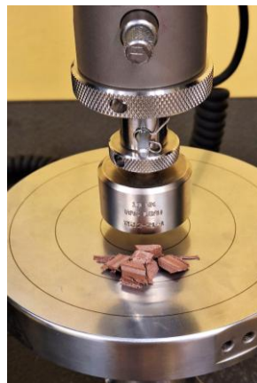
Figure 3.57. Brittle fracture during compression testing of PLA–Copper 90% specimens
