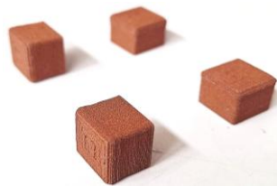
Figure 3.11. Copper Filament samples printed for compression test
