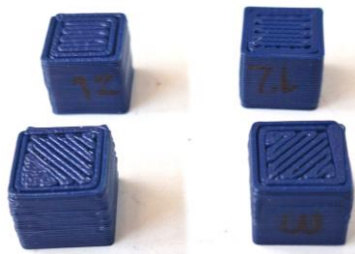
Figure 3.5. PLA samples printed for compression test
