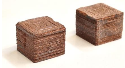
Figure 3.52. PLA–Copper 80% samples printed for compression test
