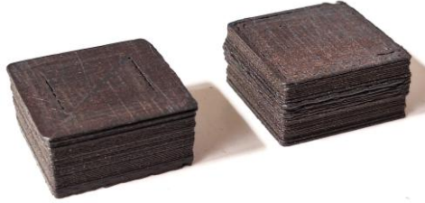
Figure 3.46. PLA–Copper 60% samples printed for thermal conductivity measurements
