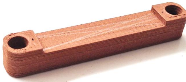
Figure 4.15. Copper Filament insert
