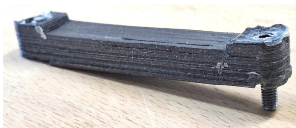
Figure 5.21. PLA–Copper 60% insert after removal from the mold
