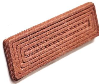
Figure 3.20. Copper Filament samples printed for DMA test
