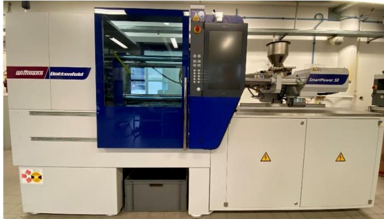
Figure 2.17. Wittmann Battenfeld SmartPower 50 injection molding machine
