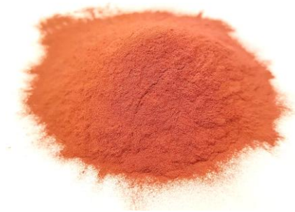
Figure 2.9. Gas atomized copper powder
