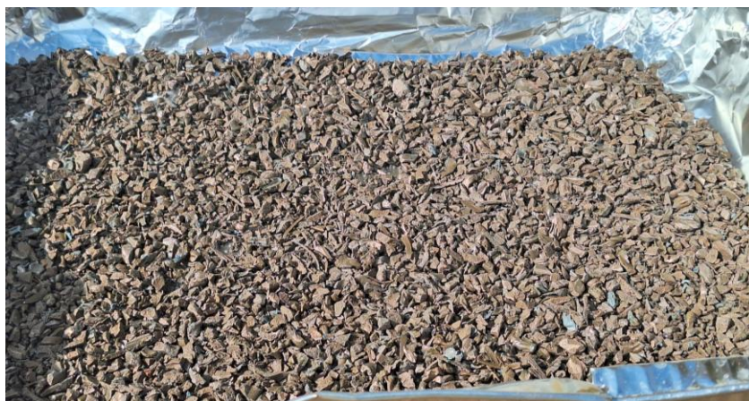
Figure 3.45. Sieved PLA–Copper composite granules
