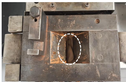
Figure 3.42. Compounding of PLA and copper using the Brabender mixer
