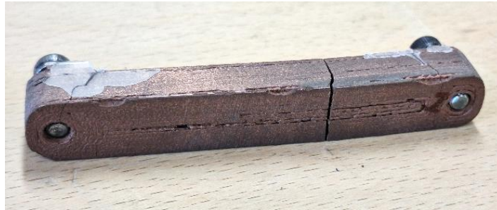
Figure 5.29. PLA–Copper 90% insert after removal from the mold
