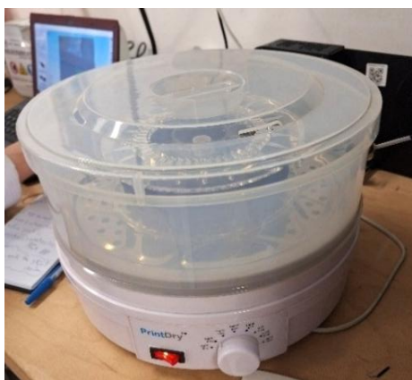
Figure 2.38. Filament Dryer – PrintDry™
