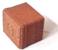
Figure 2.28. Printed specimens for compression test
