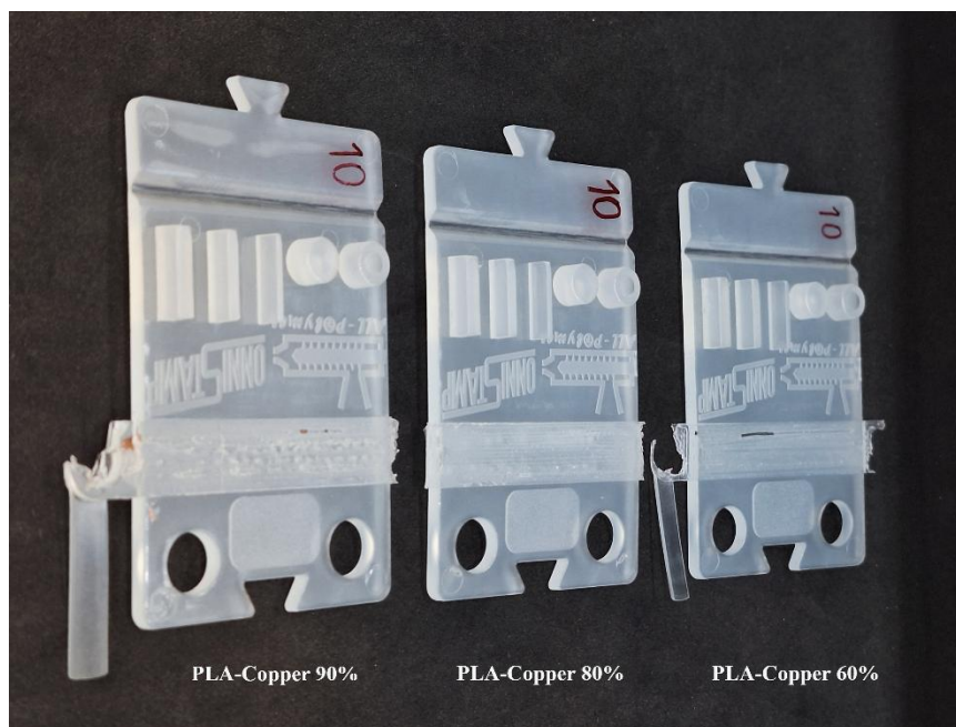
Figure 5.30. Parts molded in the 10th cycle using PLA–Copper 60%, 80%, and 90% inserts
