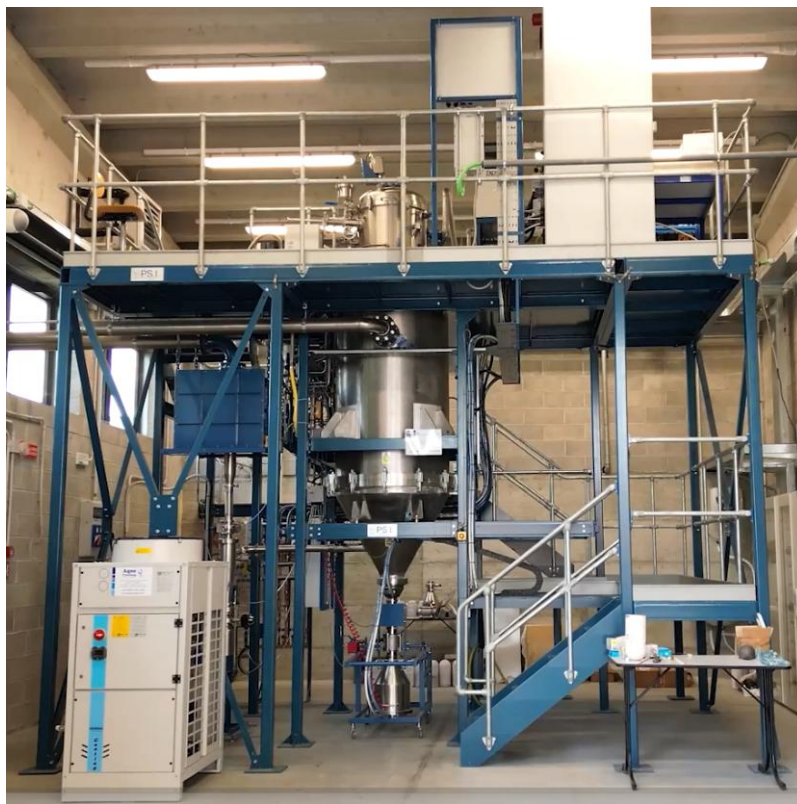
Figure 2.39. Gas Atomization system, PSI Hermiga 100/10
