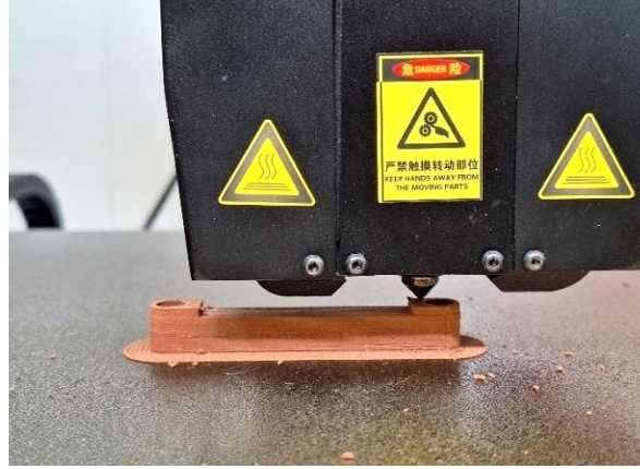
Figure 4.14. Copper Filament insert during printing with G5 PRO
