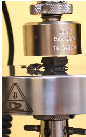
Figure 3.51. Crack propagation and fracture during compression testing of PLA–Copper 60% specimens
