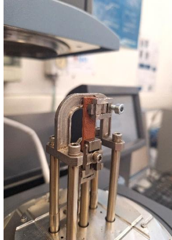
Figure 3.25. HTPLA sample printed for DMA test
