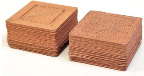
Figure 3.48. PLA–Copper 90% samples printed for thermal conductivity measurements
