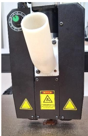
Figure 3. Manual feeding cavity used instead of the hopper
