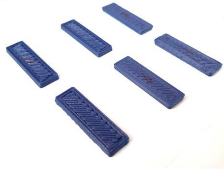
Figure 3.14. PLA samples printed for DMA test
