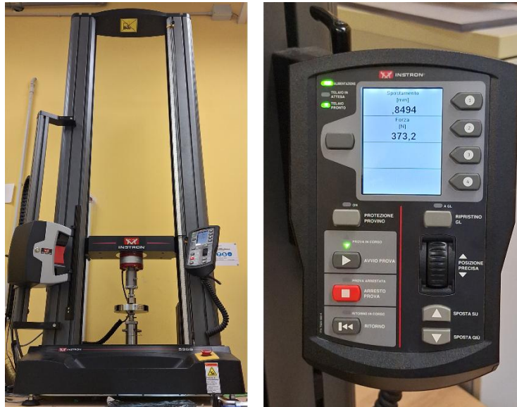
Figure 2.29. Instron 5966 Universal Testing Machine
