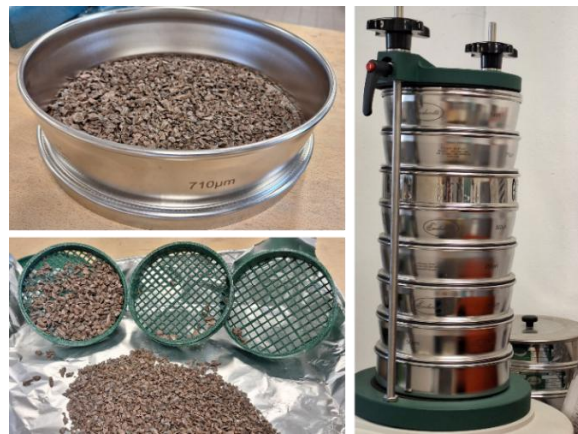
Figure 2.20. Sieves with different mesh sizes
