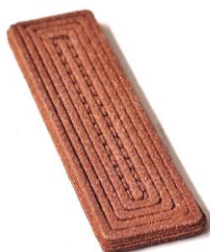
Figure 2.24. Printed specimens for dynamic mechanical analysis
