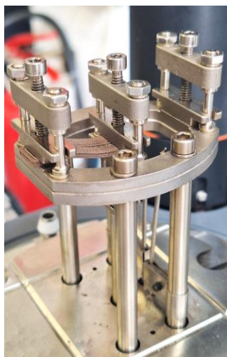
Figure 3.60. PLA-Copper 80% samples printed for DMA test
