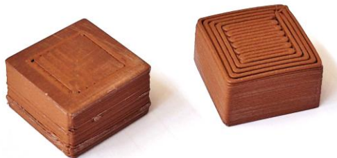
Figure 3.2. HTPLA samples printed for thermal conductivity measurements
