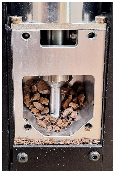
Figure 4. Screw and barrel assembly
