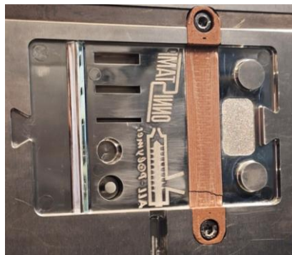
Figure 5.16. Copper Filament insert positioned inside the mold
