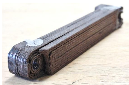
Figure 5.25. PLA–Copper 80% insert after removal from the mold
