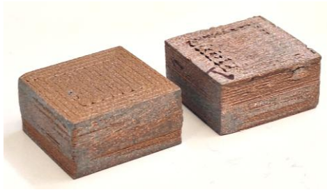
Figure 3.47. PLA–Copper 80% samples printed for thermal conductivity measurements
