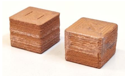
Figure 3.55. PLA–Copper 90% samples printed for compression test
