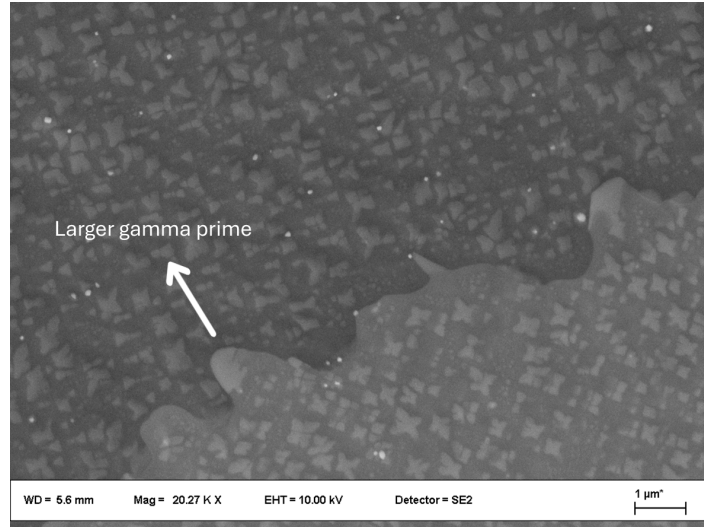
Figure 3.12: SE micrograph of the HIP sample, highlight of the grain boundary serration generated by precipitation of larger gamma prime.
