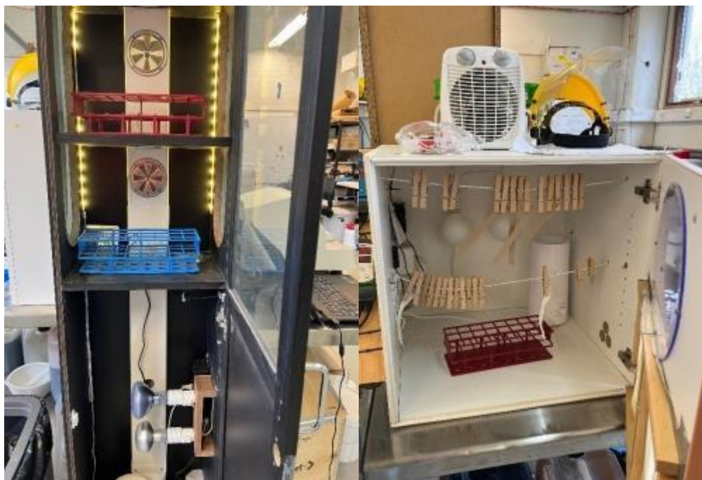
Pic 5: Climate-controlled chambers maintaining 50 \pm 2\% RH or 90 \pm 2\% RH.
