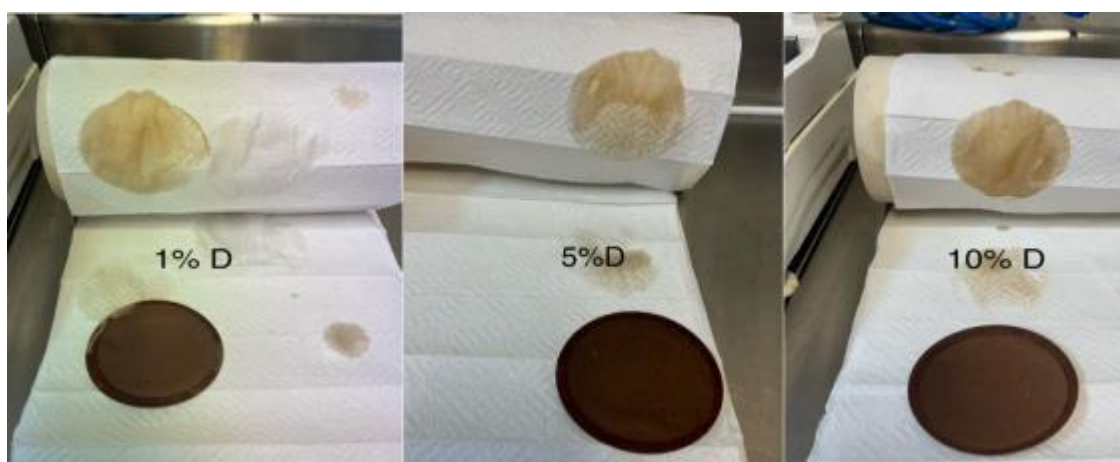
pic 10: cobb test of the dry sheet
