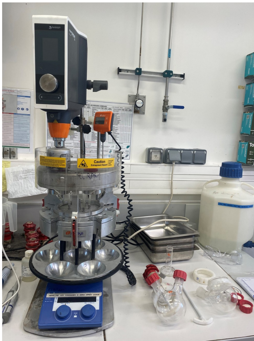
Figure 81. Tornado set up, it is possible to use more reactor at the same time and with different rotational velocity of the impeller.
