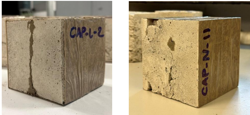
Figure 60 - Visual leakage of healing agent in different kinds of specimens
