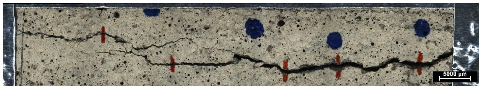
Figure 44 - CAP-L-2 crack on optical microscope observation
