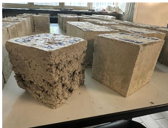
Figure 33 - Difference between a specimen with vibration defects and a properly compacted one
