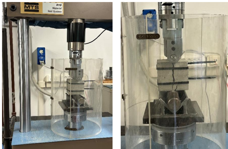
Figure 39 – Preliminary calibration for splitting test
