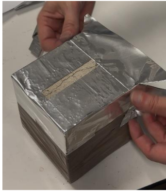
Figure 49 - Specimen preparation for absorption test
