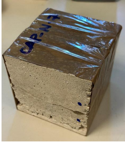
Figure 40 - Specimen wrapped in plastic tape for splitting test
