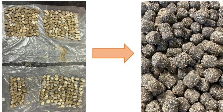
Figure 28- 5% coarse aggregate replacement by volume with CAP10 capsules
