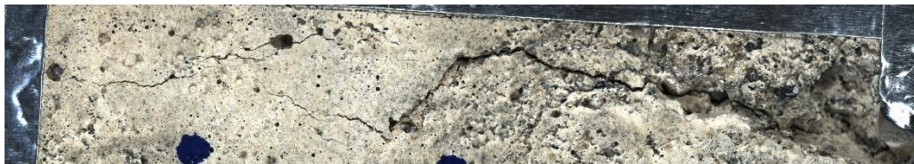
Figure 47 - Crack starting from a matrix defect
