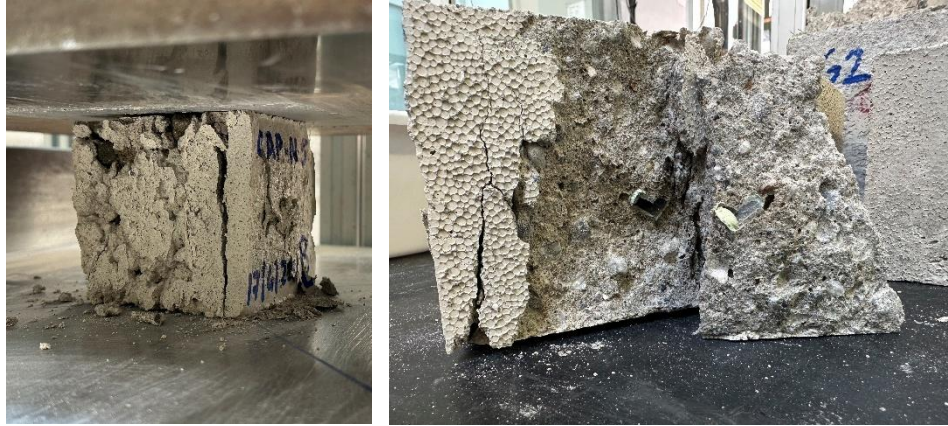
Figure 38 - Broken specimens after compressive test with capsule interception
