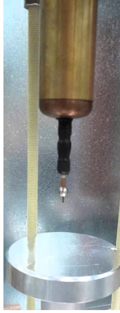
Figure 43: Point electrode used in G2Elab for breakdown experiment in air.
