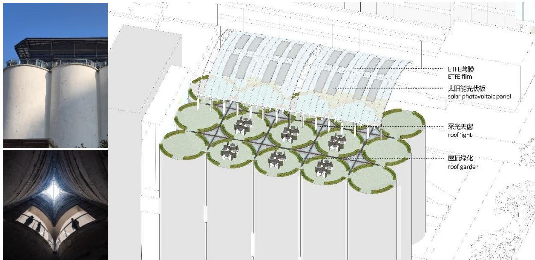
Figure 5- 28 Malt Barn Roof Reconstruction Strategy
