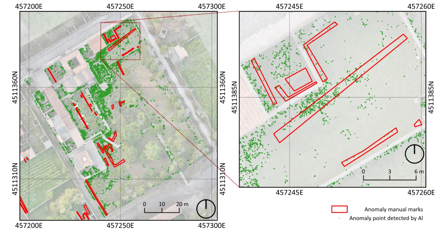
▼ Figure 154 Result of NDRE index computed through the algorithm, overlapped with the UAV map and visual interpretation
