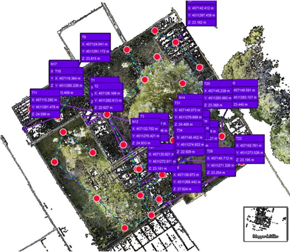
► Figure 69 Vertices used for GCP registration, with labels showing the informations
