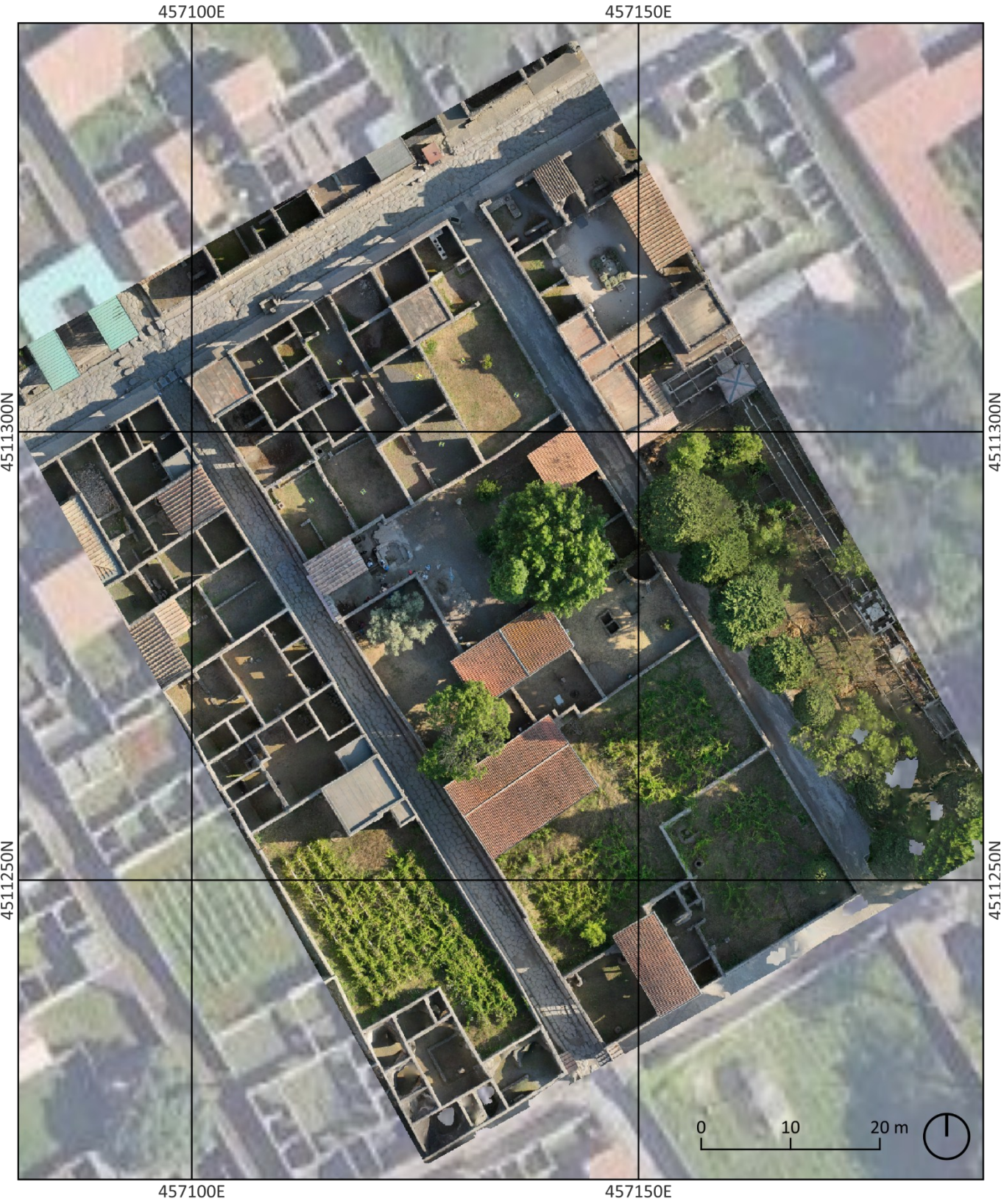
▼ Figure 75 Orthophoto of the insula Complesso Riti Magici located in, , from UAV photogrammetry
