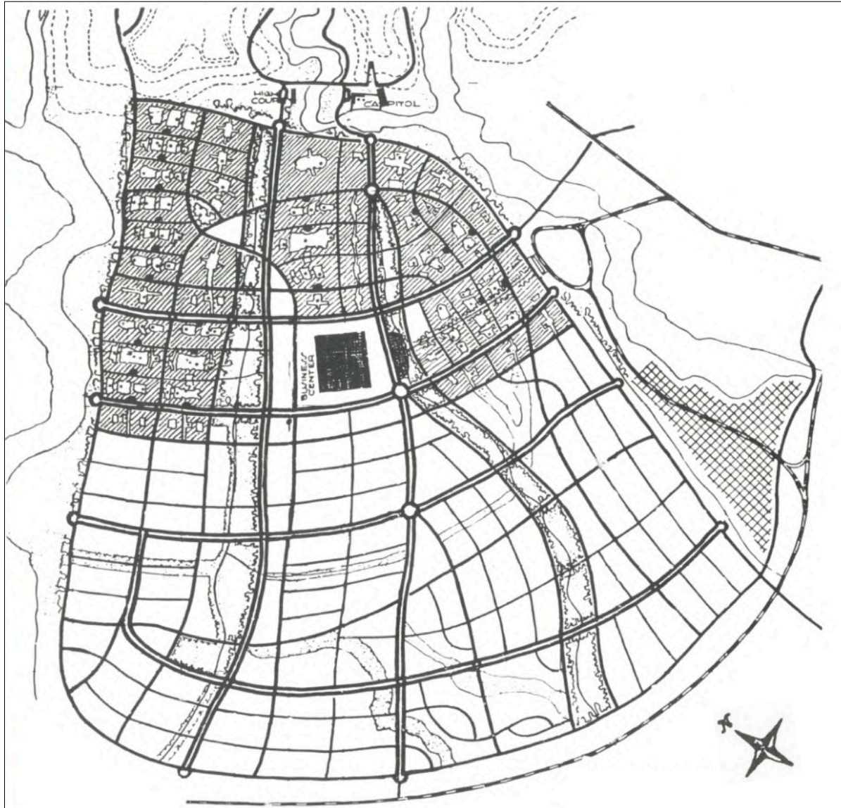
(Fig.74) The revised Albert Mayer's plan of Chandigarh, 1950 (From "Chandigarh, The Making of an Indian City" by Ravi Kalia, 1987) The black square is the city center. The idea that the city is divided into super blocks with green belts was succeeded by Le Corbusier.
