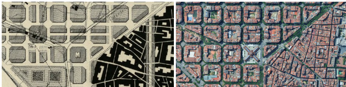
(Fig.65) Comparison of Barcelona's urban layout. (Left) A fragment of Cerdà's original plan, illustrating block types and orientations. (Right) The current state of Barcelona, where all block sides and inner courtyards have been fully built.
