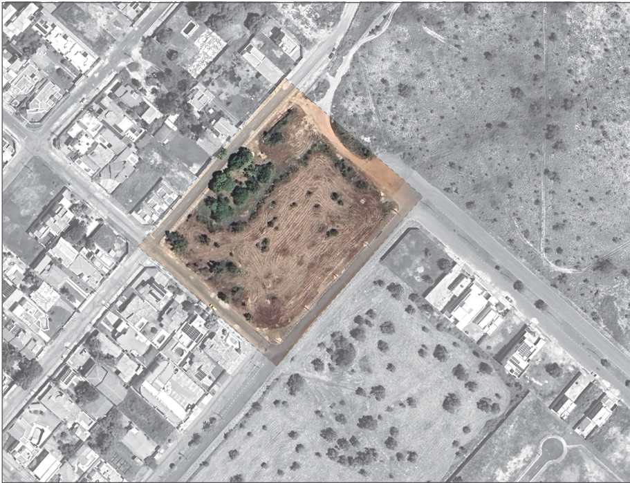
Figure 71: Design land's Properties and Dimentionss Site area - 9715 sq.m Height Restrictions - 10 meters Ground Coverage - 50% Setbacks (as per CAD plan) Coordinates - 2°51'42.0"N60°39'03.5"W
