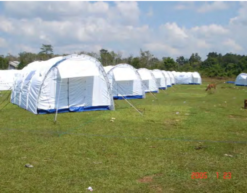
Figure 30: Above right image: The Lightweight Emergency Tent in use in Meulaboh, West Sumatra, after the Indian Ocean tsunami of 2004. The tents are arranged at an angle to prevent those in facing tents from being able to see inside when the flaps are opened. Photo by: G. Fardanesh/UNHCR
