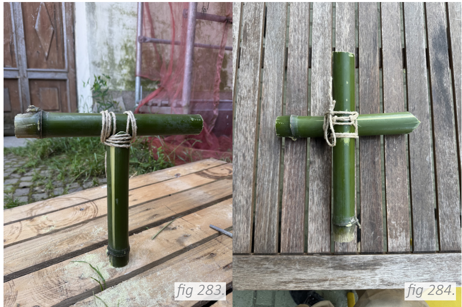
fig 283, 284. Perpendicular connection types trial with two bamboos connected with fish mouth technique (fig. 283.) and cross (fig 284.) done by the author, Photos by the author, June 30 2025.
