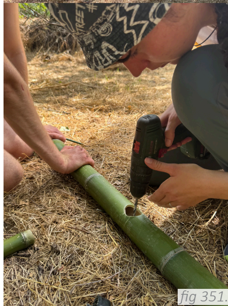
fig 351. Using a brad point drill end to align the two holes which are going to be used to insert the rows into legs, Photo by the author, July 23 2025.
