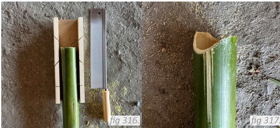
fig 316. Bamboo piece located in a Miter Box and prepared for two diagonal cut with the hand-saw.
