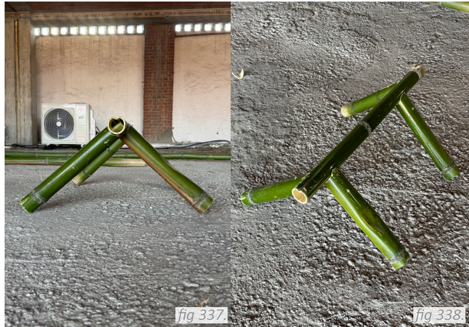
fig 337, 338. Trial product of the prototype that is basically a product of the 'Junction' technique being done four times on a single bamboo piece the legs of the structure done by the author, Photos by the author, July 4 2025.
