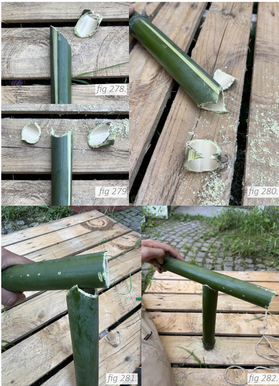
fig 278, 279, 280, 281, 282. Fish mouth connection technique trial with a machete and filing tool done by the author, Photos by the author, June 30 2025.
