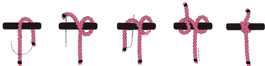
fig 375. Tying a clove hitch knot guideline for the self-building workshop, theknotsmanual.com , Drawing by the author, July 18 2025.
