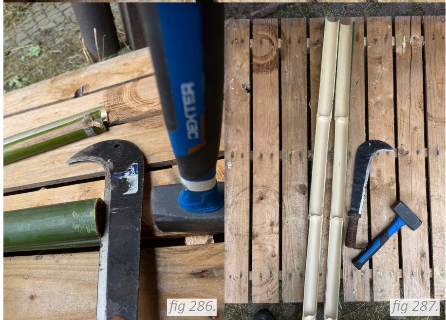
fig 286. Hitting the machete with the hammer from its back after securing the other side with a stable object. When followed the skin structure of the bamboo, it tend to be split easily and straight.
