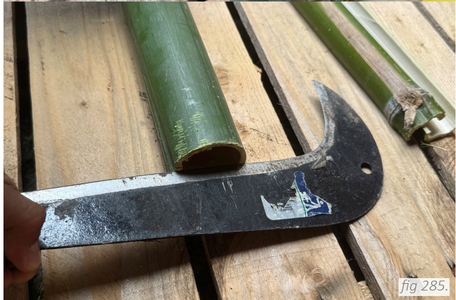
fig 285, 286, 287. Splitting the bamboo on half by using a machete and a hammer done by the author, Photos by the author, June 30 2025.
