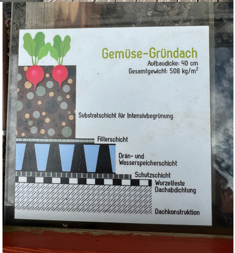
fig 202, 203, 204. Green roof simulation, showcasing its technical elements and aesthetics, Munich, Photos by the author, July 15 2024.
