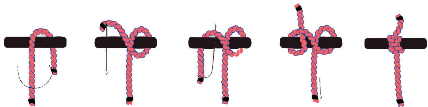
fig 362. Clove hitch knotting method, theknotsmanual.com , Scheme by the author, August 6 2025.
