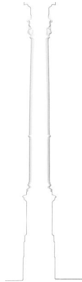
Figure 3-5 Tracing section profile from column in project
