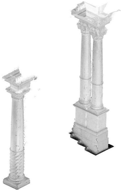
Figure 4-2 Segmented Column of Pointcloud in Atrium and in Staircase(type)
