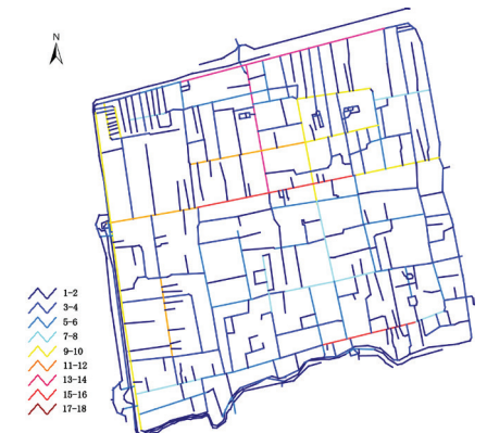
Fig 31. The space syntax graph of connectivity degree.
