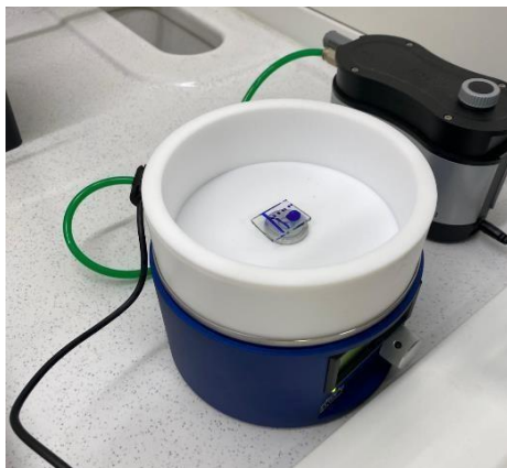
Figure 5: Spin-coater for depositing the blocking layer (source: electrochemistry lab- Polito)
