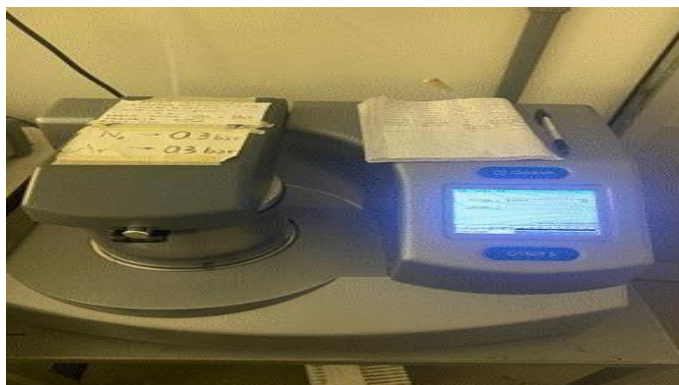
Figure 9: Platinum sputtering machine (Source: Electrochemistry Lab – Polito)
