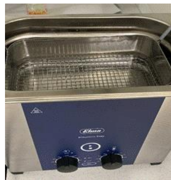
Figure 3: Ultrasonic bath used for cleaning (Source: Electrochemistry Lab – Polito)
