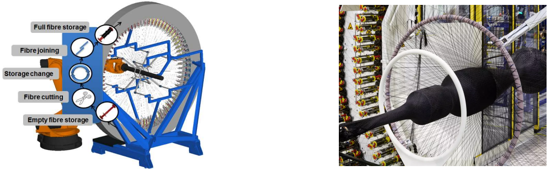
Figure 2.9: Braiding Tool Overview [52] (left), Cylindrical structure manufacture via braiding [3] (right)
