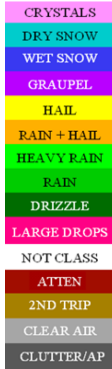
Figure 3.43: Color codes adopted by ARPA Piemonte to distinguish between hydrometeors categories when the PID algorithm is applied to the polarimetric radar variables.
