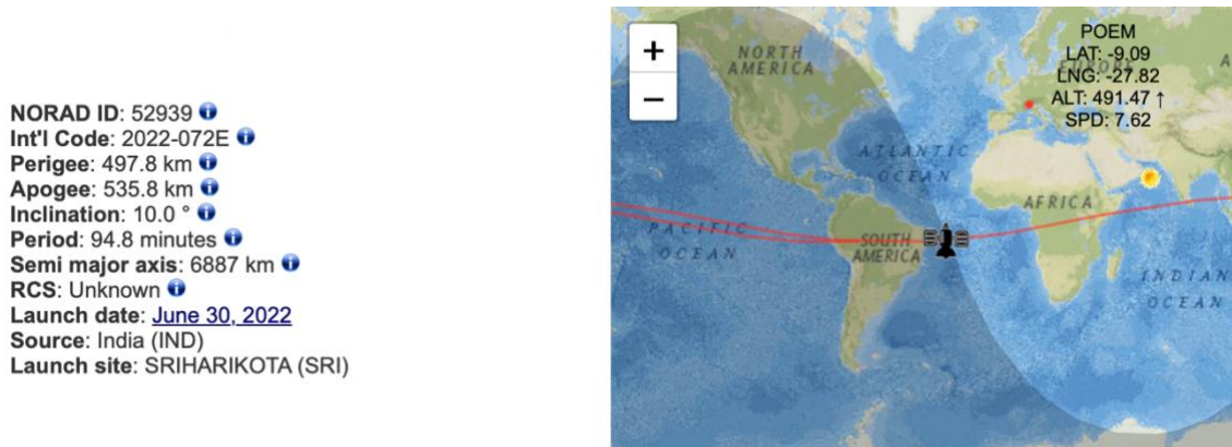
figure 15. POEM's orbital parameters and ground track
