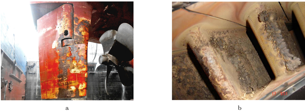
Figure 1.1: Various types of roughness: (a) Erosion along the rudder of a ship; (b) Deposition on gas turbine blades, Bons[68]
