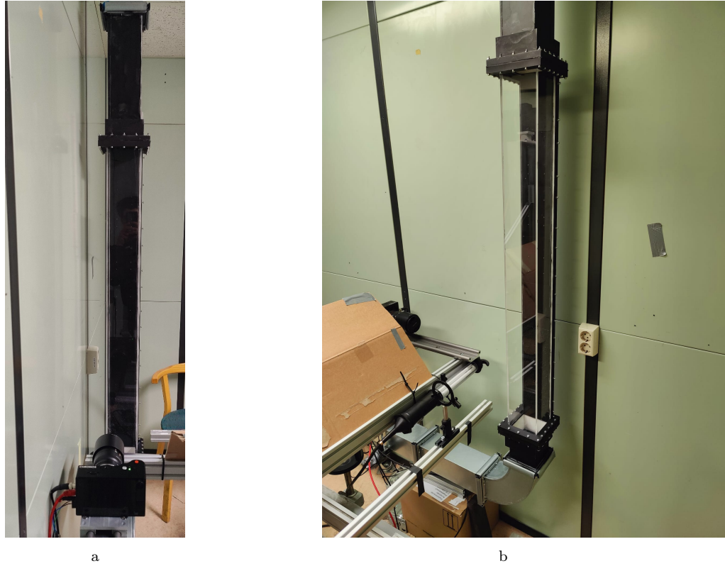
Figure 3.3: Arrangement of the test section for: (a) FULL FOV (Full Field of View) tests: Laser illuminating the plates parallel; (b) BL (Boundary Layer) tests: Laser illuminating the plates perpendicularly
