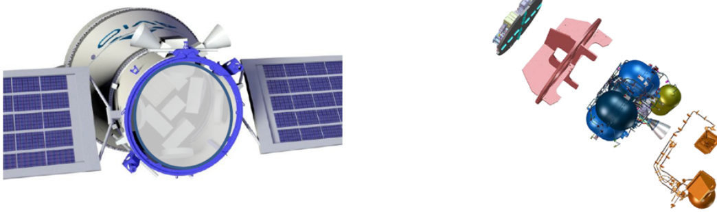
Figure 1.7: ALEK-2 render model (on the left) and AVUM+ subsystems model (on the right) [15, 16]
