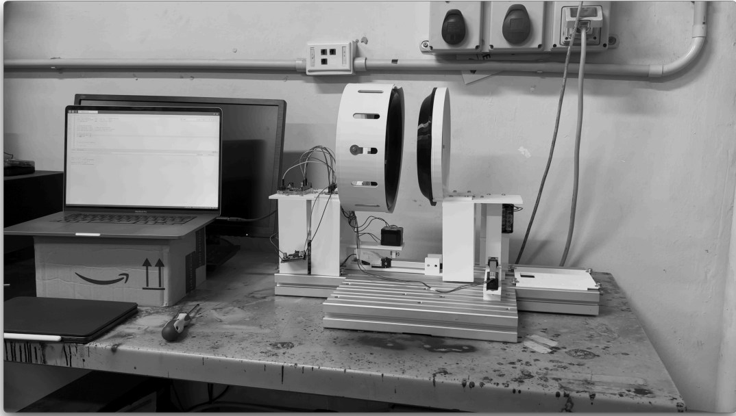
Figure 11.23: Docking test setting. Prototype (right) and PC with Arduino IDE and Serial monitor (left). The information about the test are shown on the monitor (i.e. disalignment insertion etc.)
