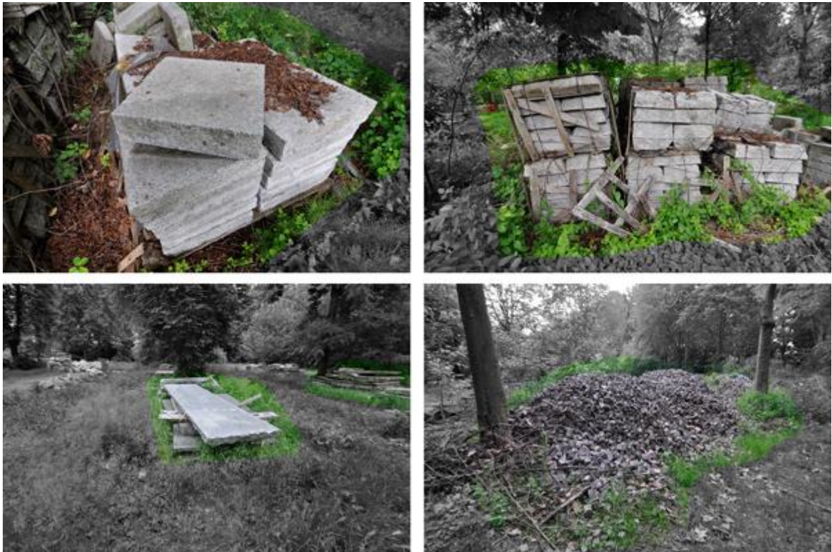
Pictures taken during April 2014 inside City warehouse of stone in Turin: granite pavers of Alzo and medium and big slabs of Luserna belongs to public space dismantling and they can be reused in the public space
