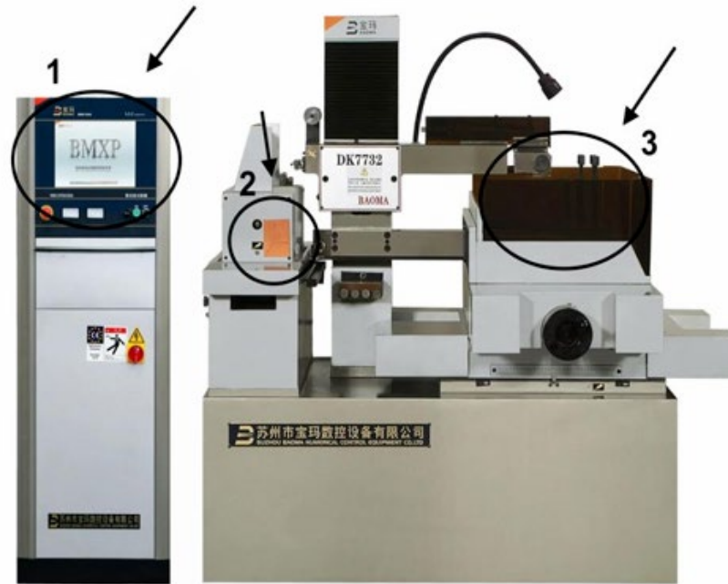
Figure 34 Key components of the WEDM machine: Section 1 (software controls), Section 2 (coordinate display), and Section 3 (cutting area).
