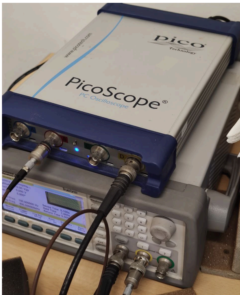
Figure 41 PicoScope and signal generator connected input/outputs
