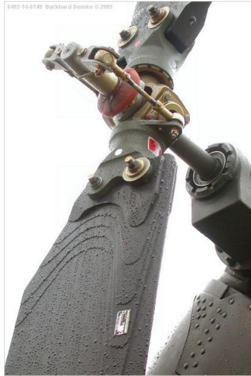
Figure 1.8 tail rotor from a Bell UH-1, with the linkages allowing the blade pitch control [23]
