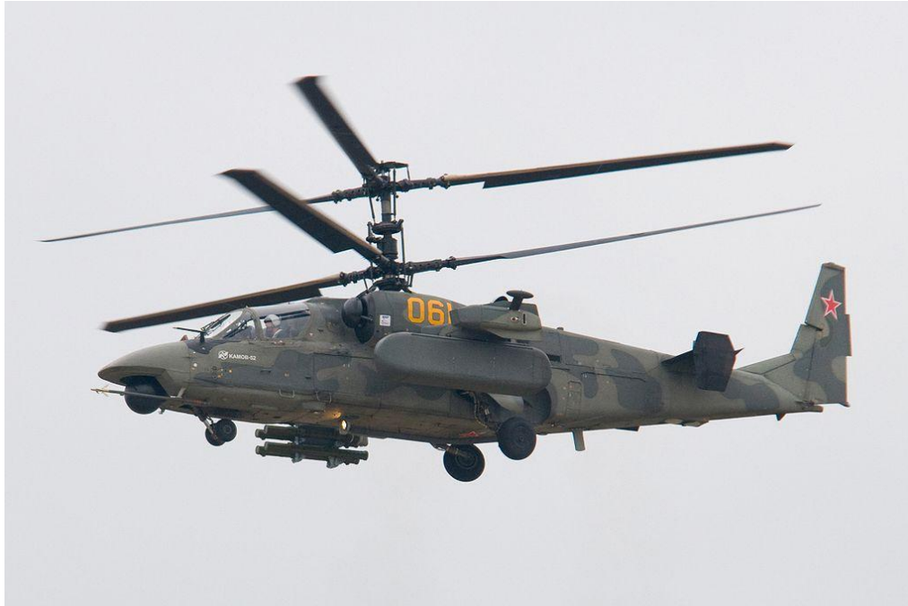
Figure 1.4 a Kamov Ka-50 featuring a coaxial main rotor [26]
