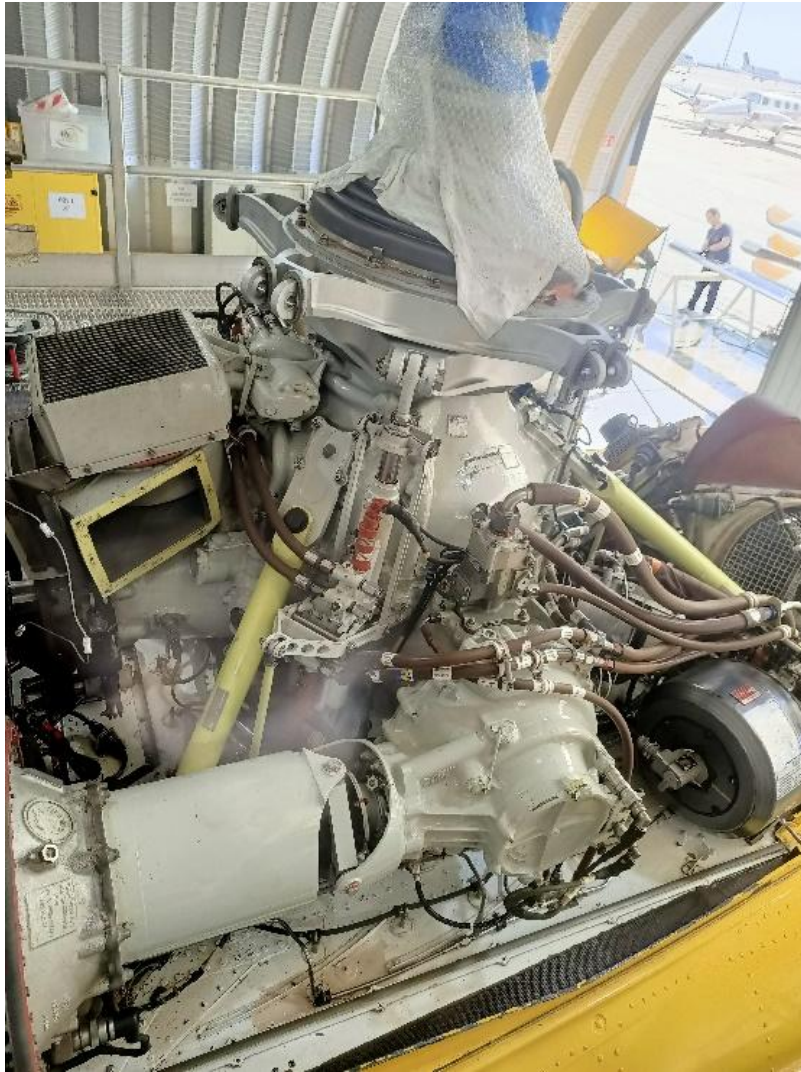
Figure 1.3 the main gearbox of a Leonardo AW139
