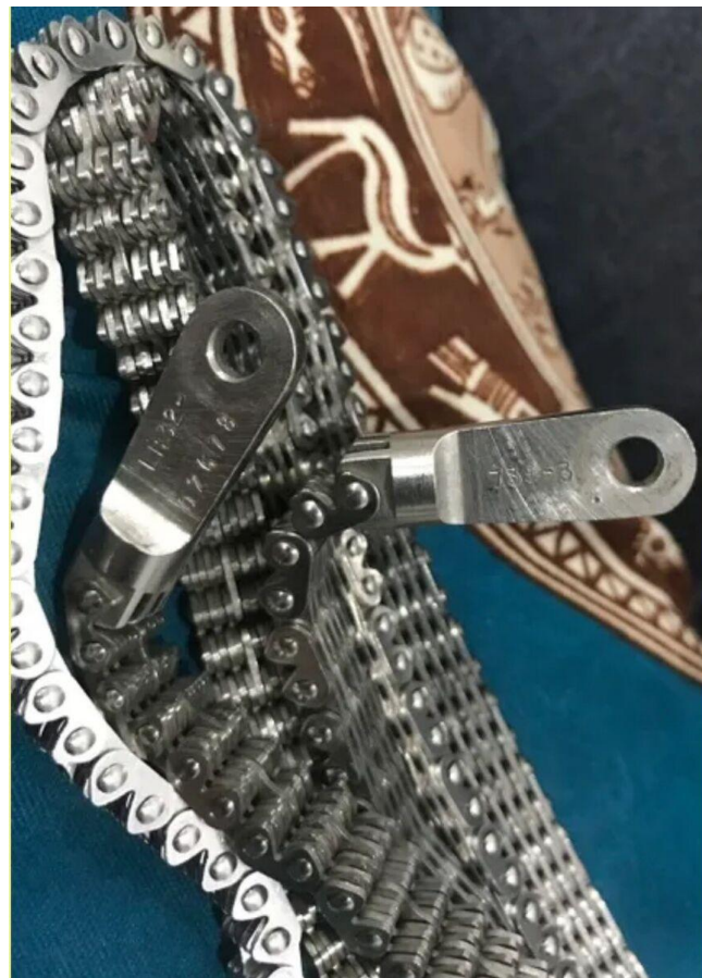
Figure 2.4 part of the pitch change mechanism control chain [29]
