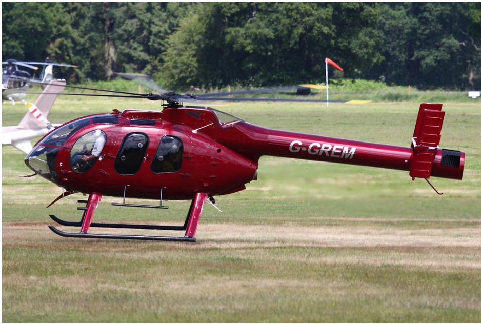
Figure 1.5 an MD-600N helicopter using the NOTAR system [24]
