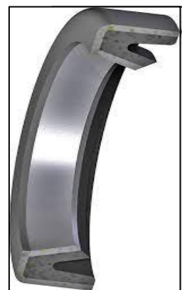
Figure 1: Three-piece radial seal cross-section. Adapted from Parker Hannifin Corporation (n.d.).
