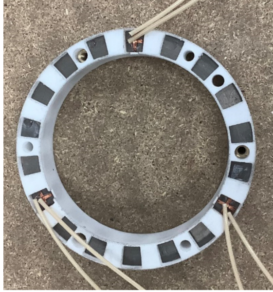
Figure 3.13: Coil windings for magnetic flux sensing installed on the carrier gear.
