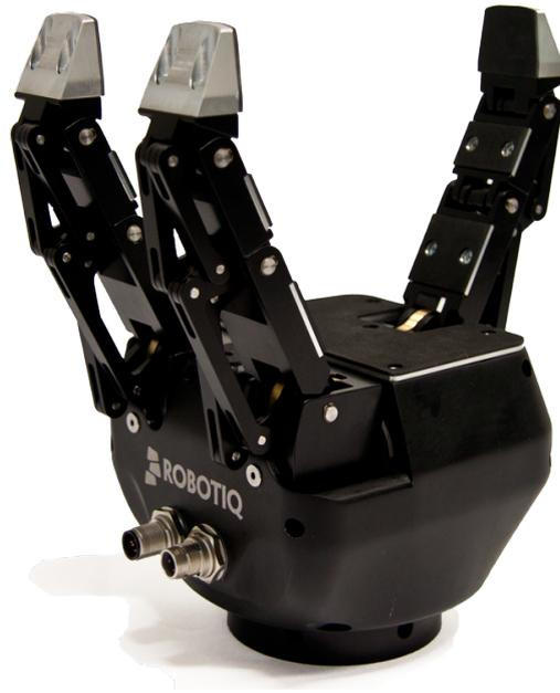
Figura 2.7 – Robotiq 3-Finger Adaptive Gripper [13]
