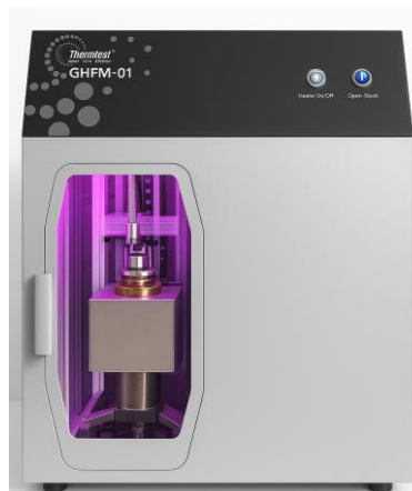
Figure 26. GHFM-01 Guarded Heat Flow Meter system for ceramic disc testing
