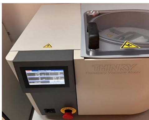
Figure 15. The THINKY Planetary Vacuum Mixer interface shows set parameters (time, speed, and vacuum) for homogenizing ceramic slurry before 3D printing
