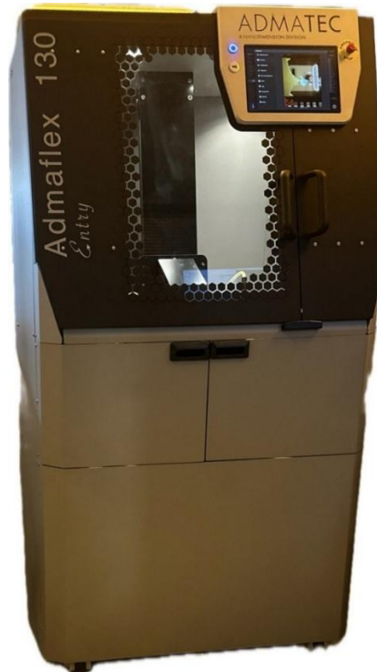
Figure 18. The Admaflex 130 Entry system is used for ceramic sample fabrication
