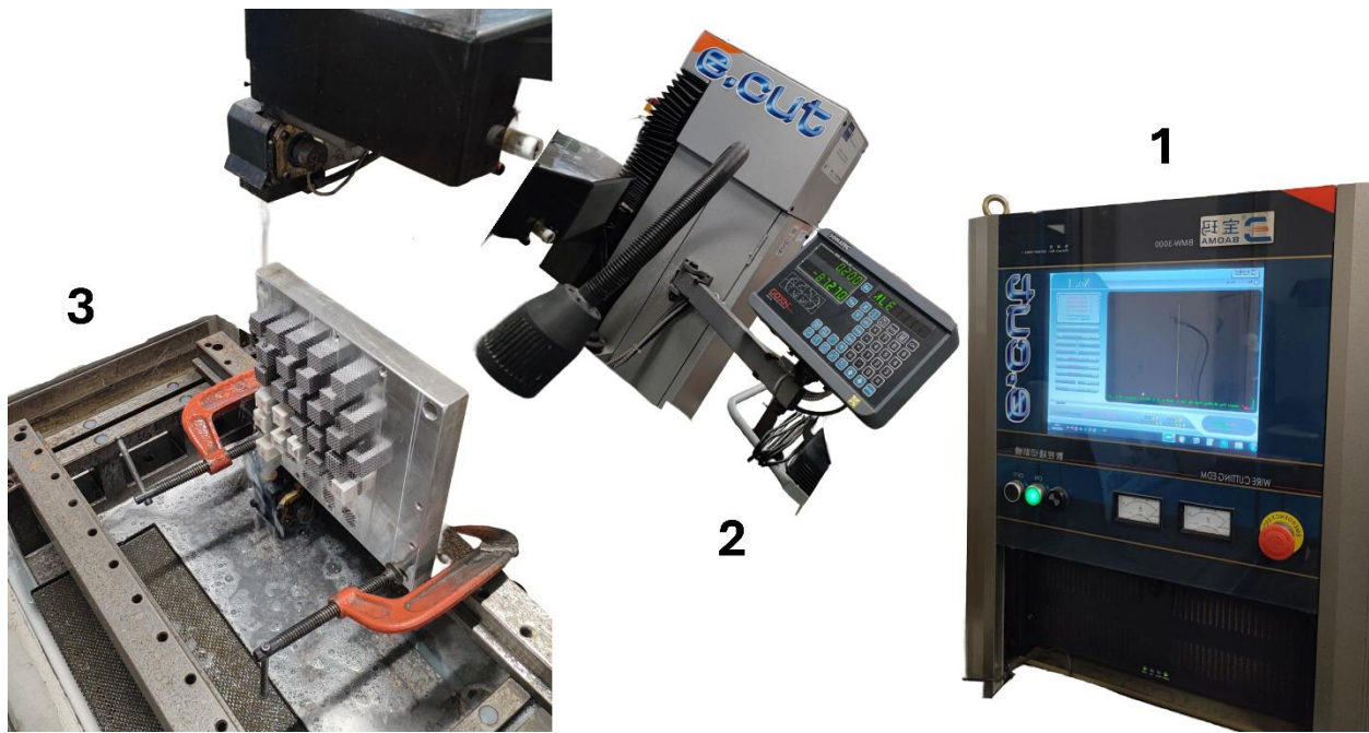
Figure 18. Key components of the W-EDM machine: Section 1 (software controls), Section 2 (coordinate display), and Section 3 (cutting area).
