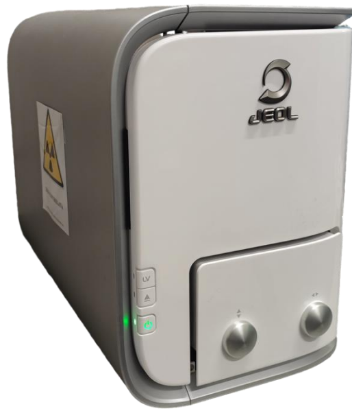
Figure 41. JCM-6000Plus SEM used for capturing fracture morphology and localized features such as crack initiation sites, delamination zones, and unfused powder particles.
